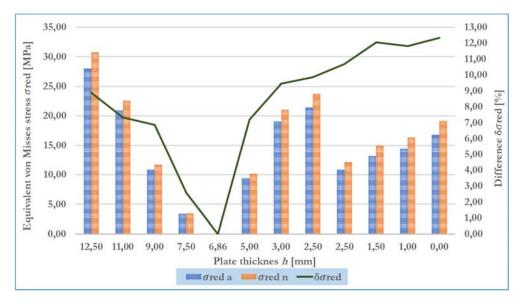
Figure 14: Comparison of equivalent von Mises stress  $\sigma_{red}$  determined analytically and numerically in the cross-section of the bimetallic perforated plate fixed and loaded with a concentrated force P = 10 kN determined on the radius  $r = R_5 = 60$  mm.
