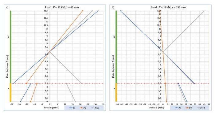
Figure 12. Stress distribution, respectively:  $\sigma_{\theta}^{"}$ ,  $\sigma_{r}^{"}$ , and  $\sigma_{red}^{"}$  in the cross-section of a bimetallic perforated plate fixed and loaded with a concentrated force with the value P = 10 kN: a) in the section T<sub>1</sub> on the radius  $r = R_5 = 60$  mm; b) in the section T<sub>2</sub> on radius r = 130 mm (Fig. 2).
