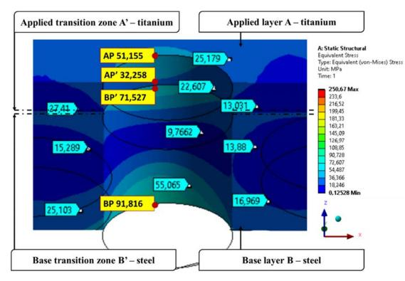
Figure 11. Distribution of equivalent von Mises stress  $\sigma_{red}^{"}$  in the cross section of the plate determined on the radius  $r = R_5 = 60$  mm.
