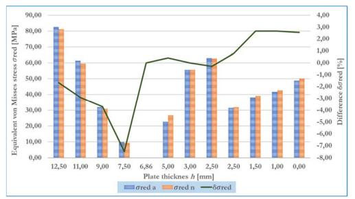
Figure 13: Comparison of equivalent von Mises stress  $\sigma_{red}$  determined analytically and numerically in the cross-section of the bimetallic perforated plate freely supported and loaded with a concentrated force P = 10 kN determined on the radius  $r = R_5 = 60$  mm.
