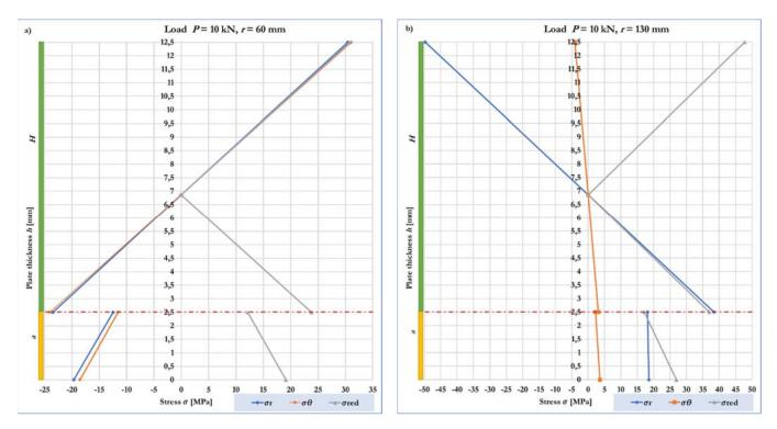
Figure 7. Stress distribution, respectively:  $\sigma_{\theta}^{a}$ ,  $\sigma_{r}^{a}$ , and  $\sigma_{red}^{a}$  in the cross-section of a bimetallic perforated plate fixed and loaded with a concentrated force with the value P = 10 kN: a) in the section T<sub>1</sub> on the radius  $r = R_5 = 60$  mm; b) in the section T<sub>2</sub> on radius r = 130 mm (Fig. 2).
