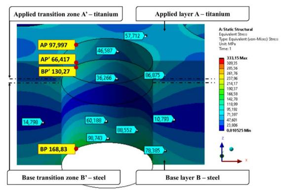
Figure 9. Distribution of equivalent von Mises stress  $\sigma_{red}^n$  in the cross section of the plate determined on the radius  $r = R_5 = 60$  mm.
