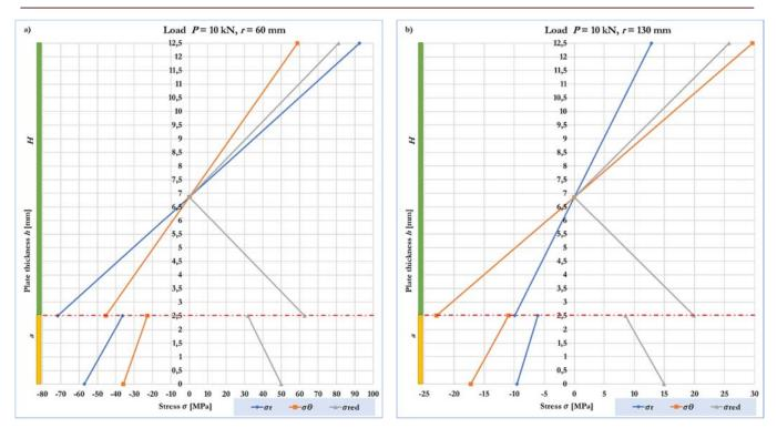
Figure 5. Stress distribution, respectively:  $\sigma_{\theta}^{a}$ ,  $\sigma_{r}^{a}$ , and  $\sigma_{red}^{a}$  in the cross-section of a bimetallic perforated plate freely supported and loaded with a concentrated force with the value P = 10 kN: a) in the section T<sub>1</sub> on the radius  $r = R_5 = 60$  mm; b) in the section T<sub>2</sub> on radius r = 130 mm (Fig. 2).
