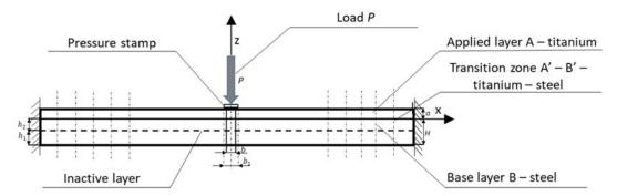
Figure 6. Bimetallic perforated plate fixed on the perimeter and loaded with a concentrated force *P* acting perpendicular to the surface In this case, the coefficients  $k_1$ ,  $k_2$ ,  $k_3$  inside the function of the lateral force intensity t(r) (6) are equal to, respectively:
