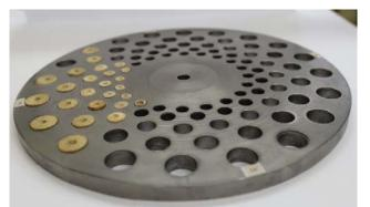
Figure 1: Model of bimetallic perforated plate.
