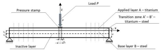
Figure 4. Bimetallic perforated plate freely supported on the perimeter and loaded with a concentrated force *P* acting perpendicular to the surface.
