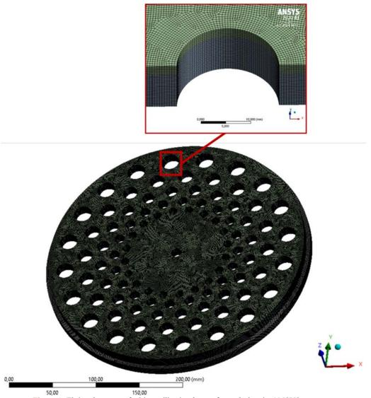
Figure 8. Finite elements of a bimetallic circular perforated plate in ANSYS program.
