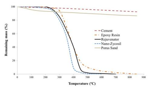
Figure 8: TGA diagrams of encapsulated ingredients.
