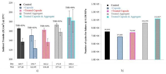
Figure 9: The results of ITS and ITF tests. a) The indirect tensile strength of specimens; b) Number of cycles required to to break specimens.
