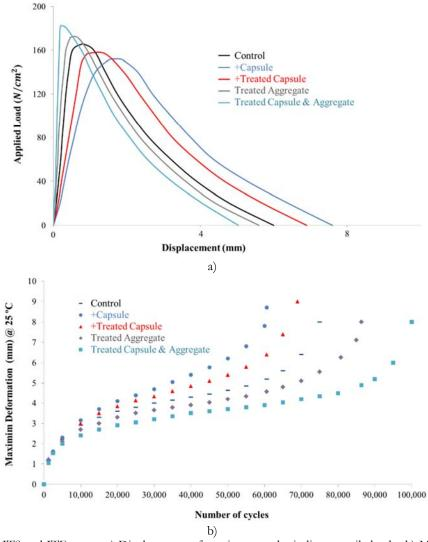
Figure 10: The results of ITS and ITF tests. a) Displacement of specimens under indirect tensile load; b) Maximum deformation of specimen during the loading Until the samples broke.
