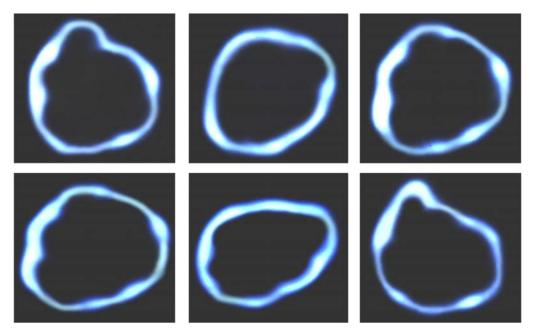
Figure 4: CT-Scan images of different capsules by shell thickness from 0.7 to 1.2 mm.
