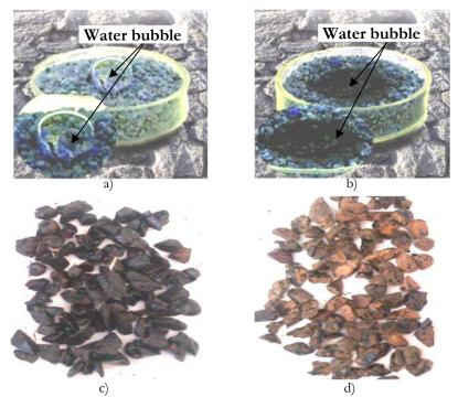
Figure 7: a) Hydrophobicity of the aggregates modified with nano-Zycosil; b) Hydrophilic in the unmodified aggregates; c) Amount of stripping in the modified aggregates (with grading according to Tab. 2); d) Amount of stripping in the unmodified aggregates (with grading according to Tab. 2).
