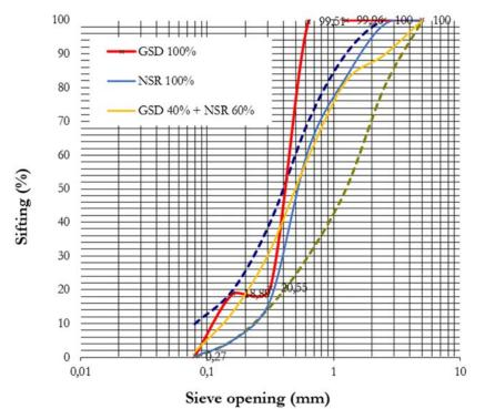
Figure 1: The grain size distribution of sands used in the experimental program.
