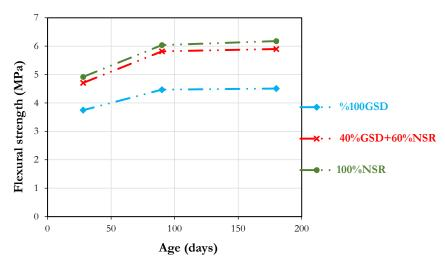
Figure 6: Flexural strength of concretes preserved in plain water in terms of age.
