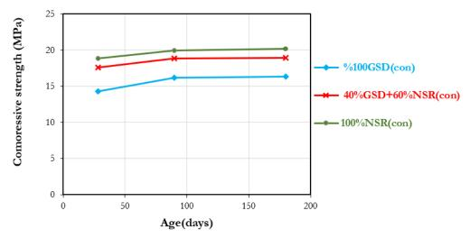
Figure 5: The effect of aggressive water on compressive strength in terms of age.
