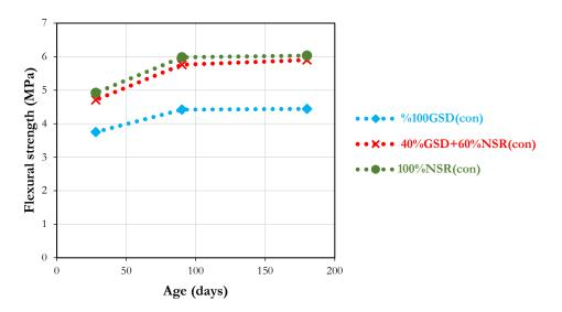
Figure 7: The effect of aggressive water on flexural strength in terms of age.
