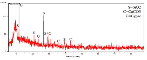
Figure 10: X-ray processing curve for Guemar Sand Dune (GSD) grains.
