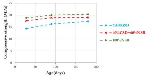
Figure 4: Compressive strength of concretes preserved in plain water in terms of age.
