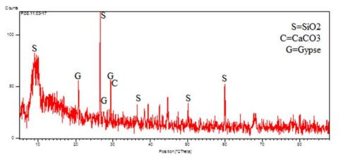
Figure 11: X-ray processing curve for Natural Sand Oued El-Ratm (NSR) grains.
