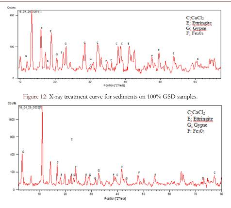
Figure 13: X-ray treatment curve for sediments on samples 40% GSD + 60% NSR.
