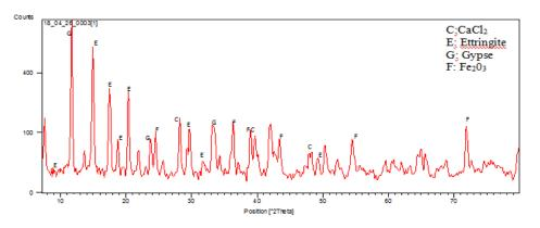
Figure 14: X-ray treatment curve for sediments on 100% NSR samples.
