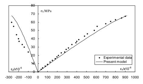
Figure 3: Simulation of stress-strain curve under uniaxial compressive test
