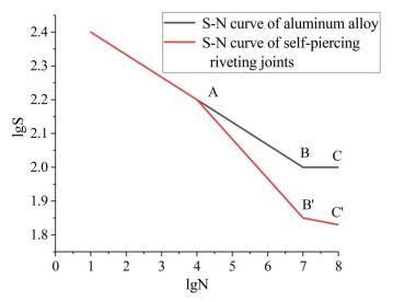
Figure 2: S-N Curve of the joints.
