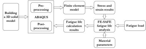
Figure 1: Flow chart of fatigue simulation analysis.
