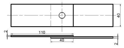
Figure 3: Size of the self-piercing riveting specimen.
