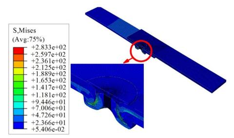
Figure 6: Stress cloud of the self-piercing riveting specimen.
