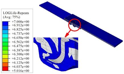
Figure 7: Fatigue simulation cloud of self-piercing riveting specimen
