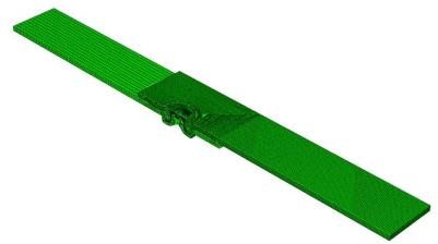
Figure 5: Mesh of the self-piercing riveting specimen.
