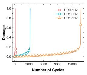
Figure 13: Fatigue damage in different notch radii (U-notched).
