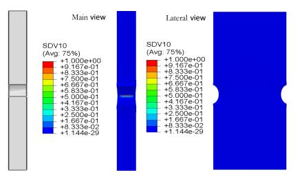
Figure 7: The fatigue damage distribution.
