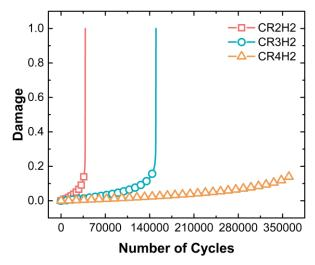
Figure 8: Fatigue damage at different root radius.
