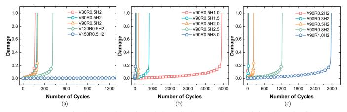
Figure 14: Fatigue damage evolution of V-notched samples: (a) notch angle, (b) notch depth, (c) notch radius.
