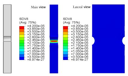
Figure 6: The plastic strain distribution.
