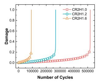
Figure 9: Fatigue damage at different root depths.
