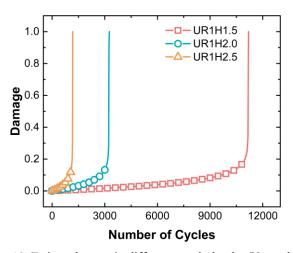
Figure 12: Fatigue damage in different notch depths (U-notched).
