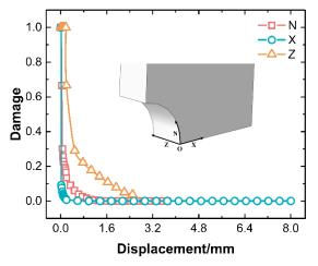
Figure 10: Fatigue damage in different directions.
