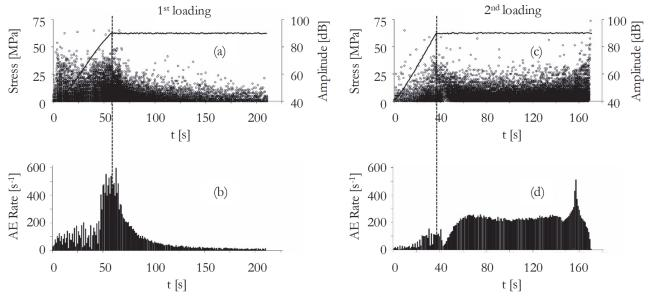
Figure 5: Time variation of (a, c) the axial stress and the corresponding amplitudes of the AE hits, and, (b, d) the corresponding behaviour of the rate of the AE hits (s<sup>-1</sup>), for the first (left column) and the second (right column) loading loop.
