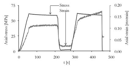
Figure 2: The time variation of the applied stress and the corresponding axial strain during the whole experimental procedure.
