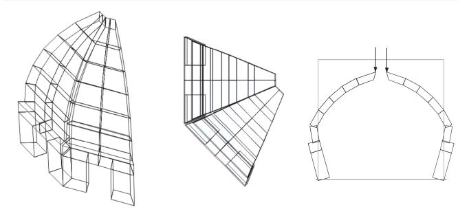
Figure 17: Collapse mechanism for case 11 (failure at ribs / Lf=2 / Nh=0 / sT=2.5 / multiplier α=13.046)
