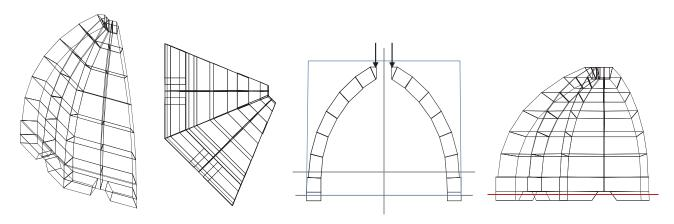
Figure 18: Collapse mechanism of S. Maria del Fiore dome (Mod1)
