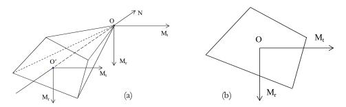
Figure 8: Yield domain. (a) The four planes through the origin O; (b) Cross section.
