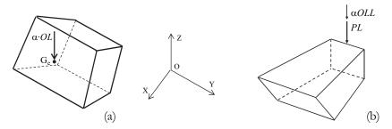
Figure 4: (a) The overload acting on the dome, increasing through an  $\alpha$  multiplier; (b) The force on the block on top corresponding to one sixteenth of the lantern own weight, together with the overload (which also increases through  $\alpha$ ) acting to the small dome of the lantern.
