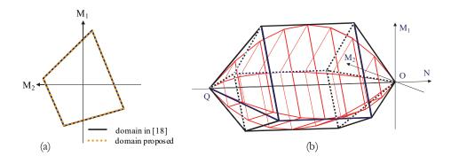
Figure 9: Yield domain for rocking in the 3D space (M<sub>1</sub>, M<sub>2</sub>, N). (a) Cross section at N=N0/2.; (b) 3D view (axonometric projection) of linearized yield domain proposed and the approximate non linear one proposed in [18].
