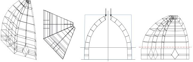
Figure 19: Collapse mechanism of S. Maria del Fiore dome (Mod2)
