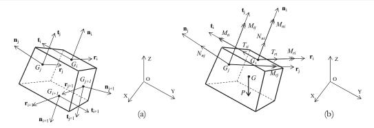
Figure 3: (a) Fixed and local references; (b) Own weight *P* acting in the *G* centroid of block and stress resultants applied on the *i* radial face and on *j* meridian face.
