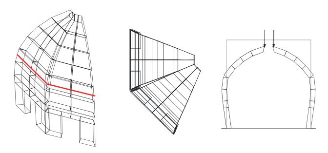
Figure 16: Collapse mechanism for case 8 (failure at ribs / Lf=2 / Nh=400 / sT=1.5 / multiplier  $\alpha$ =7.624)
