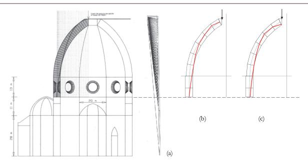
Figure 20: Comparison between our pressure curves and that of Como [19]. (a) Curve in [19]. (b) Curve obtained by imposing that it intercepts the center of the section at the drum base. (c) Curve obtained by imposing the thrust assumes the value referred in [19].
