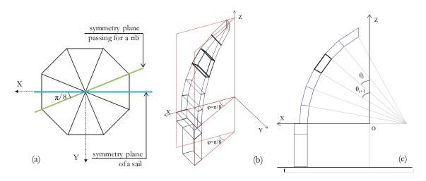
Figure 1: The dome segment. (a) the two contiguous meridian symmetry planes; (b) 3D view; (c) section in the X-Z plane.
