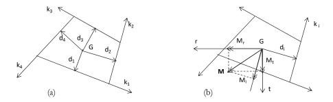
Figure 7: The quadrilateral interface. (a) Geometric aspect; (b) Mechanical aspect.
