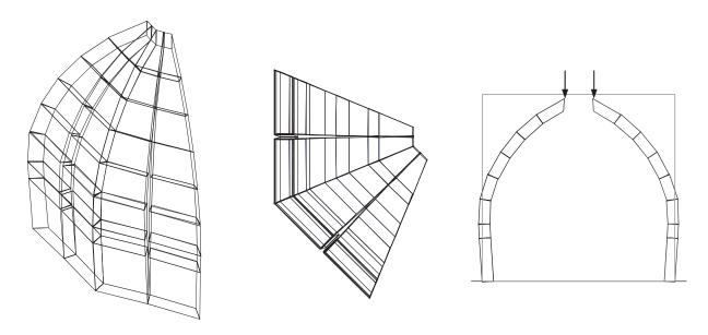
Figure 13: Collapse mechanism for case 1 (no failure at ribs / Lf=0 / Nh=0 / sT=1.5 / multiplier  $\alpha$ =24.129)
