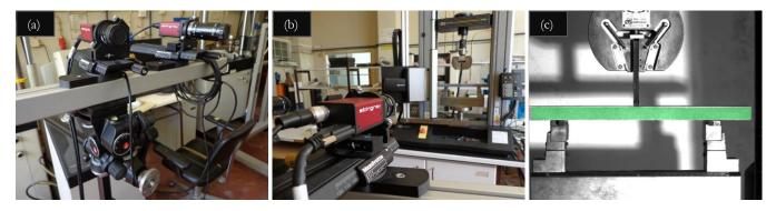
Figure 4: Digital Image Correlation with VIC2D system: (a) Cameras installation; (b) Image capturing (c) AOI.
