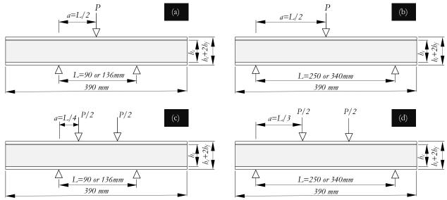
Figure 3: Schematic diagram of the test field configuration for the specimens' with: (a) 3PB short-beam; (b) 3PB long-beam; (c) 4PB short-beam; (d) 4PB long-beam. (all specimens have the same width, b=70mm, perpendicular to the paper)
