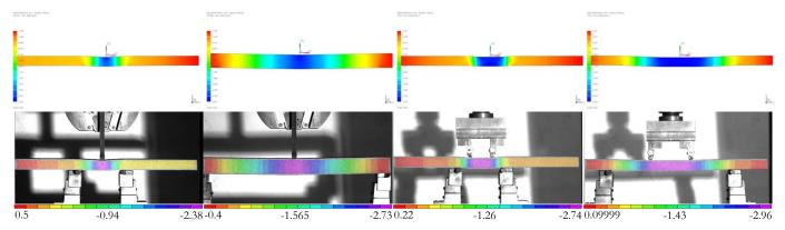
Figure 13: Mid-span *v* displacement behavior under 3PB and 4PB specimens' with 3 mm of displacement control of FEA (upper images) and DIC technique (below images) of: (a) *SB\_short\_3PB\_20*; (b) *SB\_long\_3PB\_30*; (c) *SB\_short\_4PB\_20*; (d) *SB\_long\_4PB\_20*.
