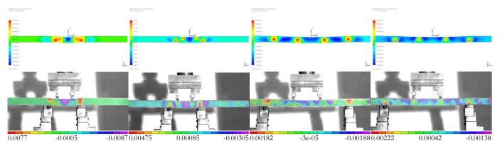
Figure 16: Mid-span  $\varepsilon_{xx}$  contour behavior under 3PB specimens' with 3mm of displacement control of FEA (upper images) and DIC technique (below images) from: (a) *SA\_short\_4PB\_20*; (b) (b) *SB\_short\_4PB\_20*; (c) *SA\_long\_4PB\_20*; (d) *SB\_long\_4PB\_20*.
