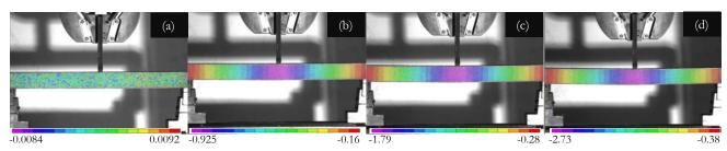
Figure 11: DIC analysis of mid-span displacement behavior of  $SB\_long\_4PB\_30$  tests with displacement control of: (a) Null; (b) 1 mm; (c) 2 mm; (d) 3 mm. (vertical displacement v [mm]).
