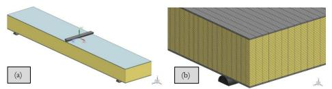
Figure 5: Finite element modelling; (a) CAD model of a 3PB long-beam specimen; (b) Detail of the FEM with uniform distribution is assumed in the faces (grey), the core (yellow) and half-cylinders (dark grey).
