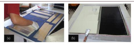
Figure 1: Manufacturing of the sandwiches with: (a) aluminum skins; (b) BFRP skins.
