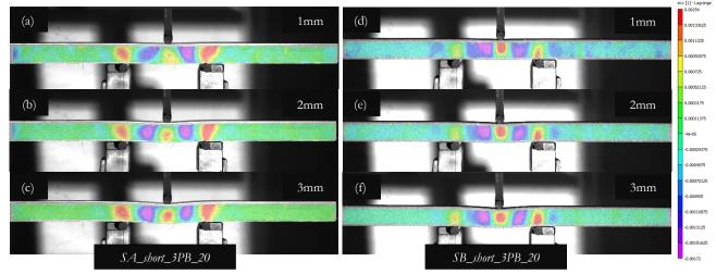
Figure 14: Mid-span VIC  $\varepsilon_{xx}$  contour behavior of: *SA* face sandwich's with (a) 1 mm; (b) 2 mm; (c) 3 mm; and *SB* face sandwich's with (d) 1 mm; (e) 2 mm; (f) 3 mm.
