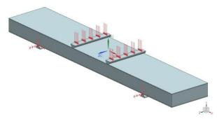
Figure 6: Example of boundary conditions on a 4PB test specimen.
