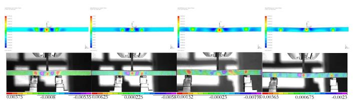
Figure 15: Mid-span  $\varepsilon_{xx}$  contour behavior under 3PB specimens' with 3mm of displacement control of FEA (upper images) and DIC technique (below images) from: (a) *SA\_short\_3PB\_20*; (b) *SB\_short\_3PB\_20*; (c) *SA\_long\_3PB\_20*; (d) *SB\_long\_3PB\_20*.
