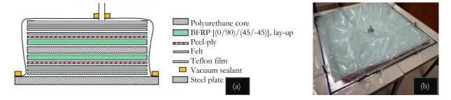
Figure 2: Manufacturing of the SB sandwich composites: (a) Stacking sequence before vacuum bagging; (b) Vacuum bag.
