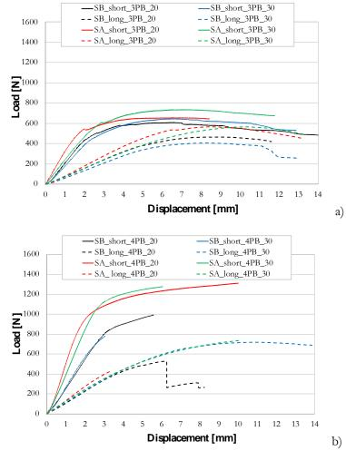
Figure 7: Load-displacement plots of sandwiches for short- and long-beam condition containing both core thickness (20 and 30mm) and for both face materials (SA and SB) under: (a) 3PB tests; (b) 4PB tests.
