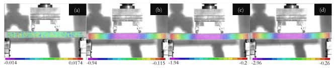
Figure 12: DIC analysis of mid-span displacement behavior of  $SB\_long\_4PB\_20$  tests with displacement control of: (a) Null; (b) 1 mm; (c) 2 mm; (d) 3 mm. (vertical displacement v [mm]).
