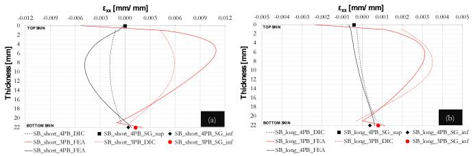
Figure 18: Mid-span  $\mathcal{E}_{xx}$  distribution for 3mm of displacement control of FEA (continuous lines \_\_\_\_) and DIC technique (dashed lines \_\_\_\_) under 3PB (red lines) and 4PB (black lines) of: (a) *SB\_short*; (b) *SB\_long* (*SG\_sup* and *SG\_inf* – refers to strain-gages in the upper and bottom faces).
