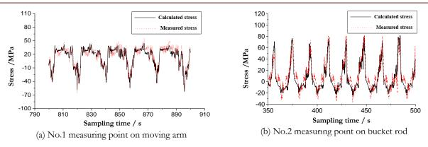
Figure 3: Comparisons of calculated stress and measured stress at measuring points
