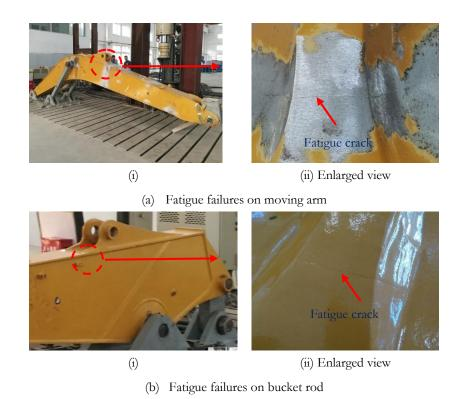
Figure 4: Fatigue failures on No.1 excavator
