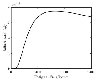
Figure 12: Failure rate curve of excavator working device
