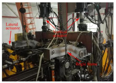
Figure 5: Platform and support mode of fatigue test
