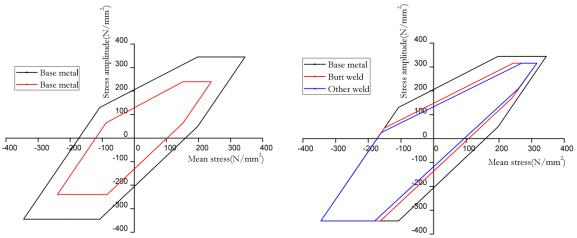
Figure 12: Comparison of Goodman-Smith fatigue limit diagrams
