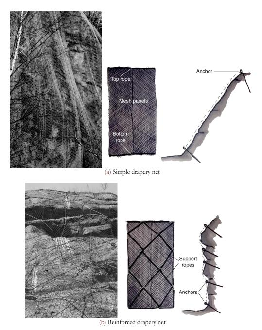
Figure 1: Views and sketches of (a) the simple drapery net and (b) the reinforced drapery net installations. Note that the reinforced drapery net follows the shape of the cliff face.
