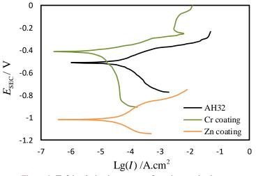
Figure 9: Tafel polarization curves of coatings and substrate
