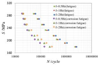
Figure 3: Results of fatigue and corrosion fatigue tests.
