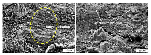
Figure 10: Morphology of crack propagation zone (a. Zn coating, b. Cr coating).
