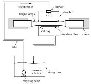
Figure 2: Setup of circulation device of corrosion solution.
