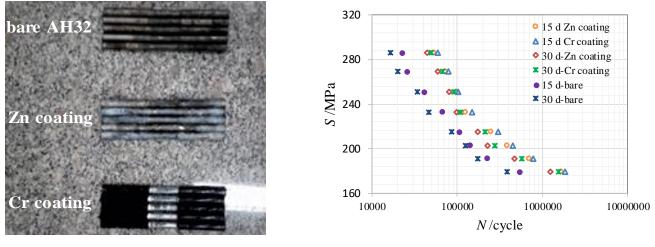
Figure 7: Morphology of the corroded samples.
