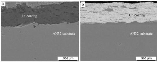
Figure 5: Cross-section microstructures of coated specimens (a. Zn coating; b. Cr coating).
