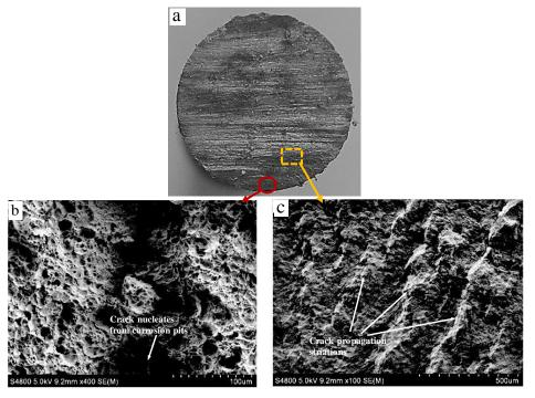
Figure 4: Fracture morphology (a. overall appearance; b. crack nucleation zone; c. crack propagation zone).
