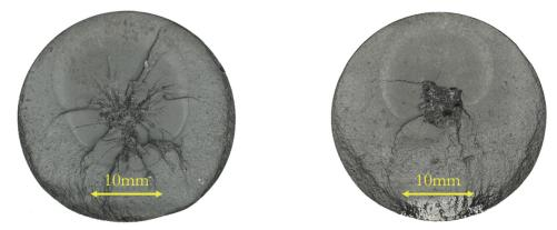
Figure 5: Fracture surface of a FT#A defect (specimen "GP1") (a) and of a FT#B defect (specimen "GP21") (b)
