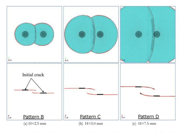
Figure 4: Fatigue crack growth behavior of two non-coplanar embedded cracks. The horizontal separation S of the initial crack tips is 10 mm, and the vertical height H is (a) 2.5 mm, (b) 5.0 mm and (c) 7.5 mm. Only crack shape is displayed. The red line shows the crack tip. The top figure is the top view of the crack shape, and the bottom figure is the front view of the crack shape. The crack growth behavior is categorized into (a) pattern B, (b) pattern B, and (c) pattern B, respectively.
