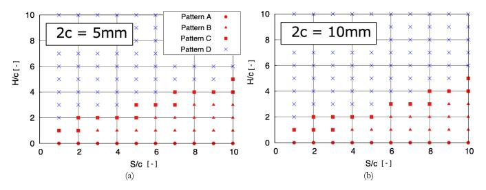
Figure 7: Interaction map of two non-coplanar embedded cracks obtained by the s-FEM simulations. The initial crack sizes are (a)  $2\iota = 5$ mm and (b)  $2\iota = 10$ mm. The plot is based on the length of H and S normalized by the half size of crack  $\iota$ . The borders determined by the JSME and Ando et al. are also plotted.
