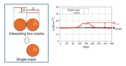
Figure 8: Stress intensity factor distribution along the crack tip of two non-coplanar embedded cracks. The stress intensity factor increases near the other crack. The position along the crack tip is denoted with the angle theta defined in the figure (left). In order to study the interaction of two embedded cracks, the stress intensity factor of a single embedded crack is also calculated.
