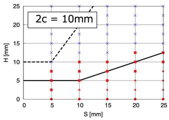
Figure 6: Interaction map of two non-coplanar embedded cracks obtained by the s-FEM simulations. The initial crack size is 2e=10mm. The plot is based on the real length of H and S. The borders determined by the JSME and Ando et al. are also plotted.
