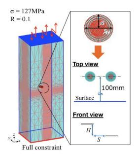
Figure 2: Finite element mesh for the fatigue crack growth simulation of two non-coplanar embedded cracks. Each cracks is modelled with each local mesh separately. The position of the center of two cracks are at 100 mm distance from the surface of the specimen. The horizontal separation and vertical height of the crack tips are denoted by H and S. The maximum tensile stress is 127 MPa, and the stress ratio R is 0.1. The displacement at the bottom surface is fully constraint.
