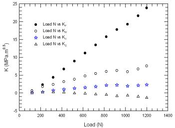
Figure 4: Stress intensity values given by the mixed-mode CJP equation, with  $K_F$  defined perpendicular to the 45° slant crack and  $K_{II}$  defined parallel with the slant crack in the CT specimen.
