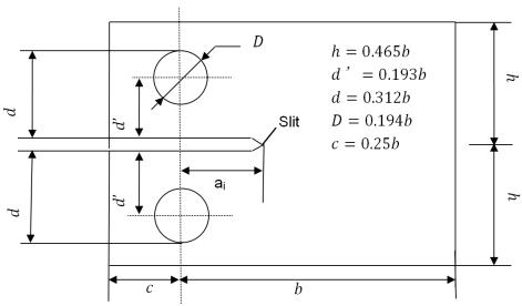
Figure 2: Geometry and dimensions (in millimetres) of the polycarbonate compact tension (CT) specimens used in this work. Note that the notch length (equal to the initial crack length)  $a_i = 20$  mm and the width b = W = 72 mm are defined from the centreline of the holes.
