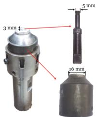
Figure 10: FSW tool used
