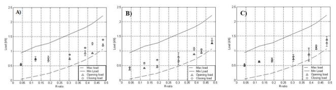
Figure 7: A) Illustration showing the variation of the opening and closing loads with the R-ratio for a 42 mm crack using a horizontal strain gauge, B) a 45° strain gauge, C) a back face strain gauge.
