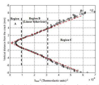
Figure 3: Graph of showing the linear relationship between the vertical distance from the crack tip and  $(S_{max})^{-2}$  employed in the methodology of Stanley and Chan for the calculation of the stress intensity factor from thermoelastic data.
