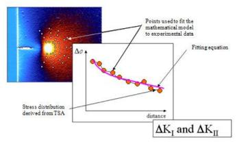
Figure 4: Schematic illustration of the methodology for calculating the stress intensity factor from thermoelastic data.
