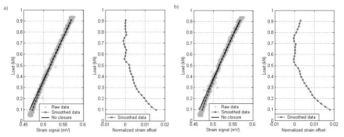
Figure 6: Illustration showing load vs. strain and load vs. strain-offset plots for a 42 mm crack in an aluminium CT specimen loaded between 0.94 and 0.04 kN (R-ratio 0.04). a) Unloading branch. b) Loading branch.
