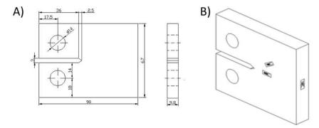
Figure 5: A) Illustration the dimension of aluminium CT specimens employed for fatigue tests; B) Scheme showing the location and orientation of the strain gauges employed for the calculation of the opening and closing loads from the compliance traces
