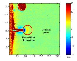
Figure 2: Typical phase map for a 6mm fatigue crack. Illustration of the phase shift occurring at the crack tip as a result of the loss of adiabatic conditions (dimensions in mm).
