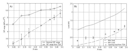
Figure 8: A) Plot showing the variation of  $\Delta K$  with the R-ratio for a sequence of thermoelastic images corresponding to a 42 mm crack. B) Plot illustrating the variation with the R-ratio of the opening load inferred from a sequence of thermoelastic images.
