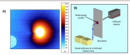
Figure 1: A) Typical thermoelastic pattern of a fatigue crack. B) Schematic illustration of the calibration process.
