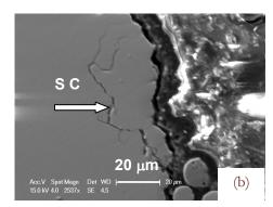
Figure 5: (a) Cracking surface for the specimen tested in water, at  $\sigma_{max}$ =156 MPa and  $N_{f}$  =8× 10<sup>7</sup>, (b) secondary cracking (SC) in the cross section of the specimen tested in 3.5% NaCl, at  $\sigma_{max}$ =41.3 MPa and  $N_{f}$  =9× 10<sup>7</sup>.
