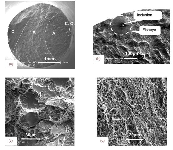
Figure 3: Fracture surface of a specimen tested in laboratory air, at  $\sigma_{max} = 610$  MPa and  $N_f = 3.27 \times 10^8$ , (a) whole fracture surface (C.O.: crack origin), (b) enlargement of Region A, (c) enlargement of Region B and (d) enlargement of Region C.
