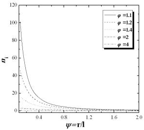
Figure 6: Predicted *n*<sub>i</sub> of subsurface crack initiation for specimens tested in air, for different loading levels and material properties.
