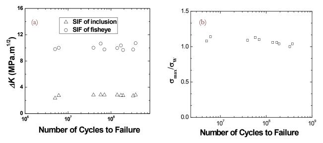
Figure 4: (a)  $\Delta K$  for inclusions and fisheyes, (b) relationship between  $\sigma_{\text{max}}/\sigma_{\text{w}}$  and number of cycles to failure.
