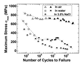
Figure 2: S-N curves for specimens tested at laboratory air, fresh water and 3.5% NaCl aqueous solution, hollow symbols: crack origination at surface, solid symbols: crack origination at subsurface, semi-solid symbols: mixed crack origination.
