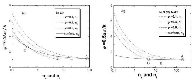
Figure 7: (a) Predicted results of fatigue life for surface and subsurface crack initiation in air, (b) predicted S-N curves for surface and subsurface crack initiation in 3.5% NaCl solution.
