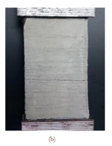
Figure 8: (a) Micro-crack bridging and ductility enhancement effect of PVA fibers; (b) Typical multiple cracks on ECC thin plate specimen under tensile load.
