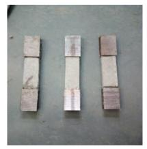
Figure 3: The thin Plate Specimen for uniaxial compression experiment.
