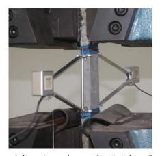
Figure 4: Experimental set-up for niaxial tensile test.
