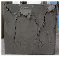
Figure 1: Failure mode of test specimens.
