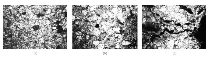
Figure 3: The structures of the cross sections of the samples for three different values of D and at the same thickness of explosive charge – 5 mm: a) D=3.19 km/s; b) D=3.95 km/s; c) D=5.26 km/s.
