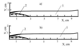
Figure 8: Compacted and destruction regions for various explosive thicknesses under external pressures P = 0.05 Mbar (a) and P = 0.075 Mbar (b). The detonation velocity is D = 5 km/s. The solid, dashed, and dot-and-dash lines refer to the explosive thicknesses  $\delta_c = 2$  cm,  $\delta_c = 3$  cm, and  $\delta_c = 5$  cm, respectively. The compacted and destruction regions are indicated by 1 and 2.
