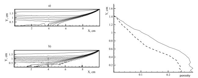
Figure 9: Density isolines for  $\delta_{\epsilon} = 0.5$  cm: a) cylindrical configuration; b) planar statement.
