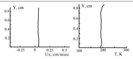
Figure 18: Distributions of the longitudinal velocity  $u_x$  (a) and temperature T (b) across the compacted region of the sample for the detonation velocity D = 3 km/s.
