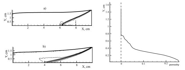
Figure 11: Density isolines for  $\delta_{\epsilon} = 1$  cm: a) cylindrical configuration; b) planar configuration.
