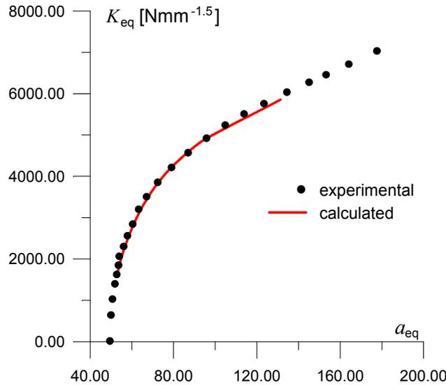
Figure 10: Comparison between calculated and experimental R-curve.
