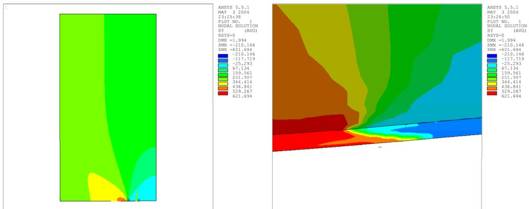
Figure 11: Calculated stress distribution in the traction direction (y) for  $\Delta a = 25$  mm.
