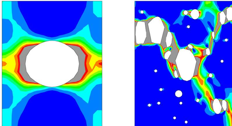
Figure 2: Equivalent strain distribution inside two RVE.
