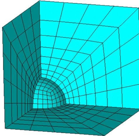
Figure 4: FE model of the single void cell.
