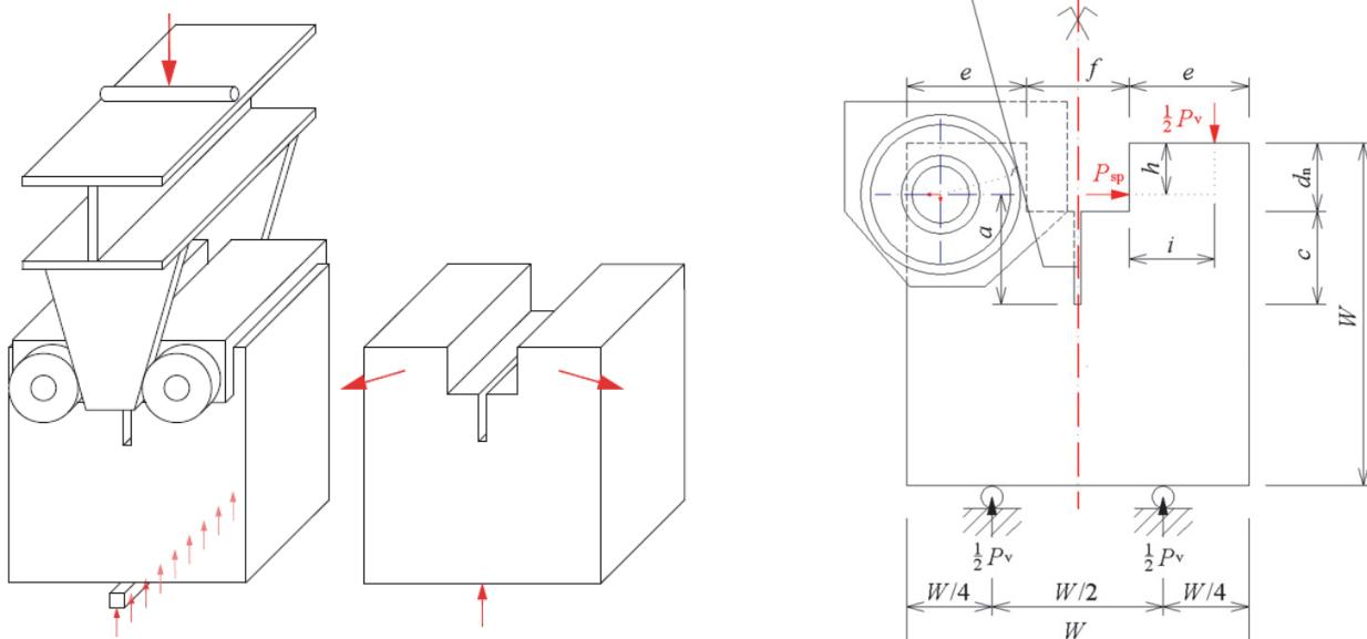
Figure 1: Wedge splitting test with the schema of loading imposition (left); geometry of the analysed wedge splitting test specimen (right)[15].
