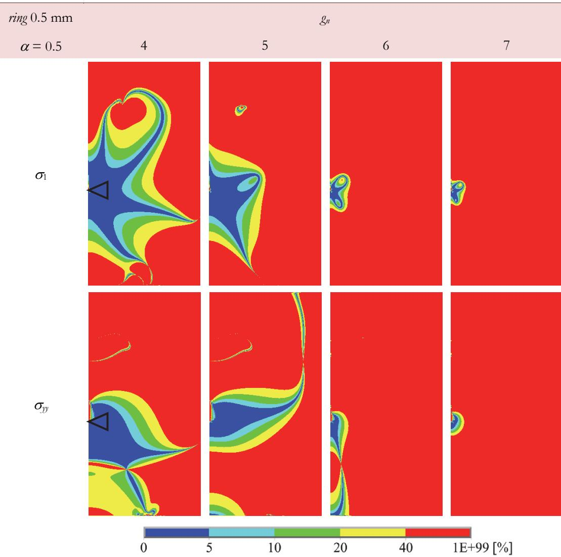
Figure 8: Progress of relative error of the  $\sigma_1$  and  $\sigma_{yy}$  reconstruction with increasing number of Williams series terms used.
