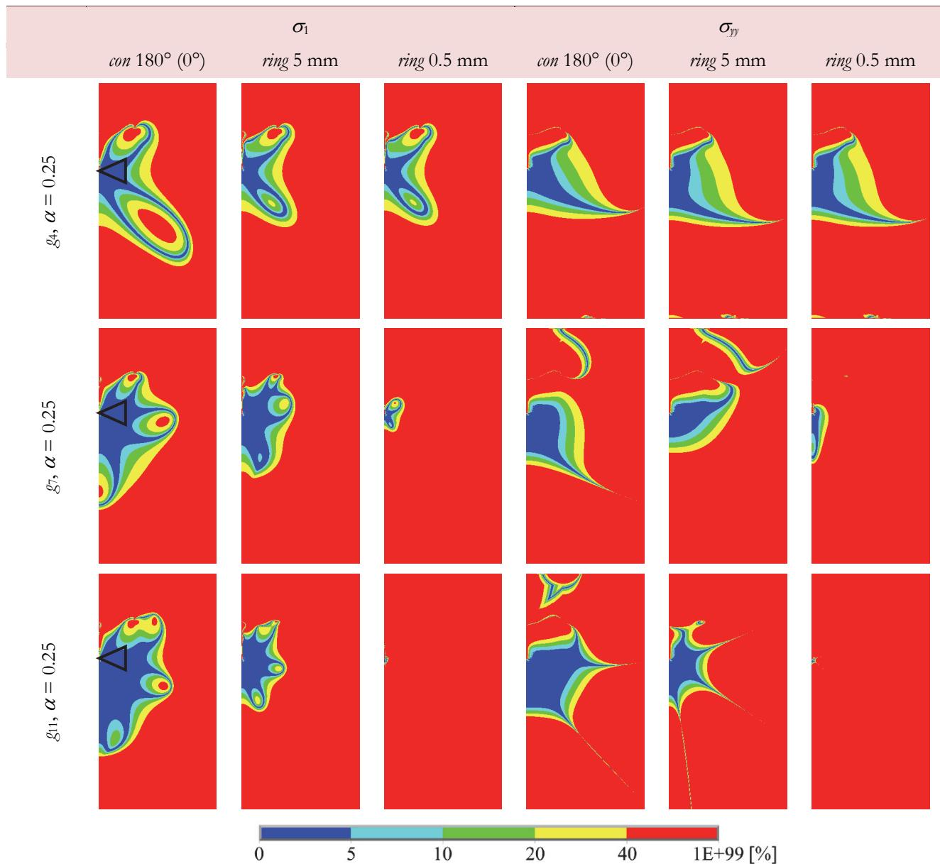
Figure 9: Progress of relative error of the  $\sigma_1$  and  $\sigma_{yy}$  reconstruction for selected terms of Williams series used.
