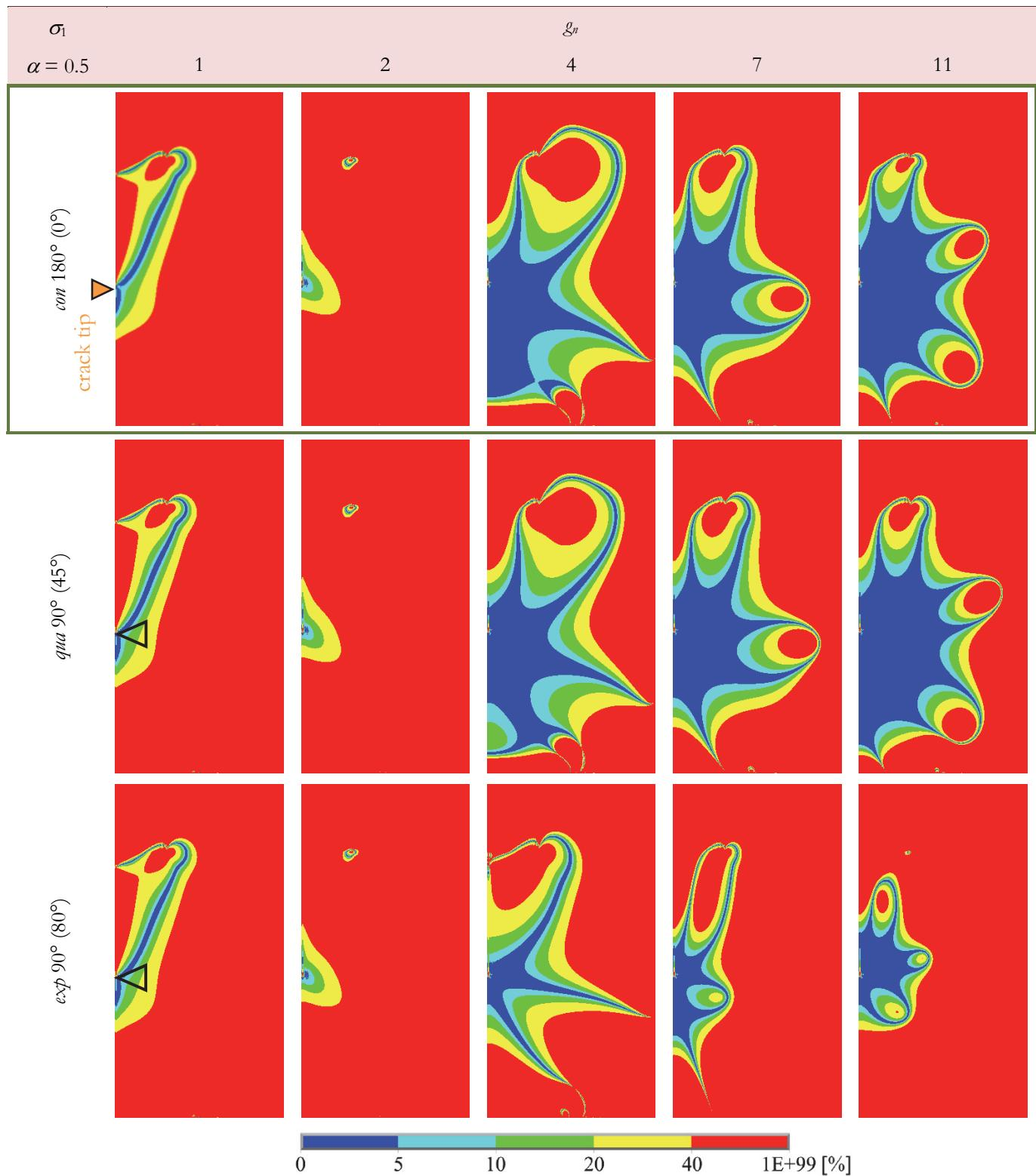
Figure 4: Relative error of principal tensile stress  $\sigma_1$  field approximation for chosen variants of nodal selection.
