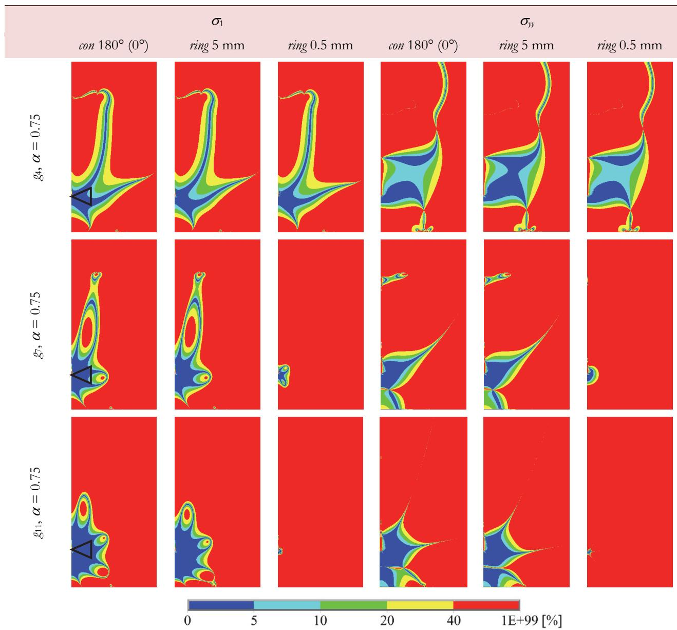
Figure 10: Progress of relative error of the  $\sigma_1$  and  $\sigma_{yy}$  reconstruction for selected terms of Williams series used.
