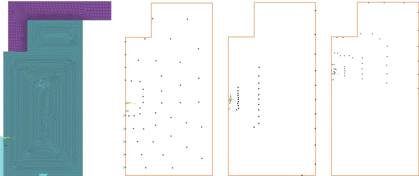
Figure 3a: Numerical model of the WST specimen, used finite element mesh [22].
