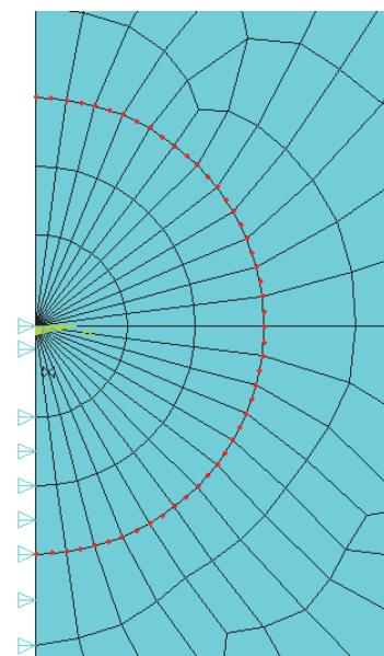
Figure 2c: Detail of the FE mesh for the ring 0.5 variant with nodal selection (red dots at the distance 0.5 mm from the crack tip).
