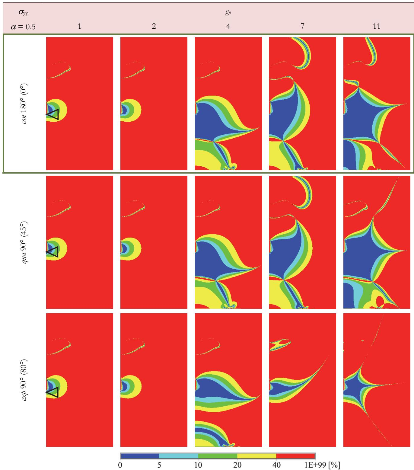
Figure 5: Relative error of crack opening stress  $\sigma_{yy}$  field approximation for chosen variants of nodal selection.
