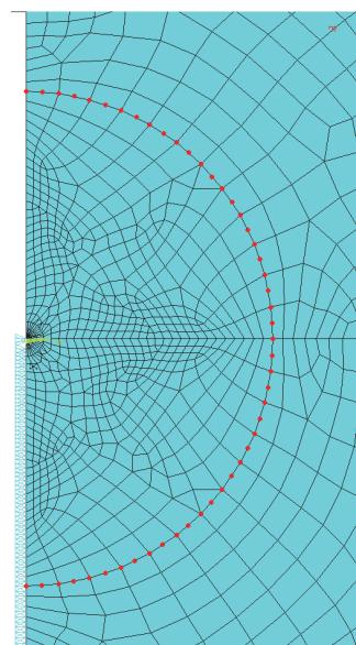
Figure 2b: Detail of the FE mesh for the ring 5 mm variant with nodal selection (red dots at the distance 5 mm from the crack tip).
