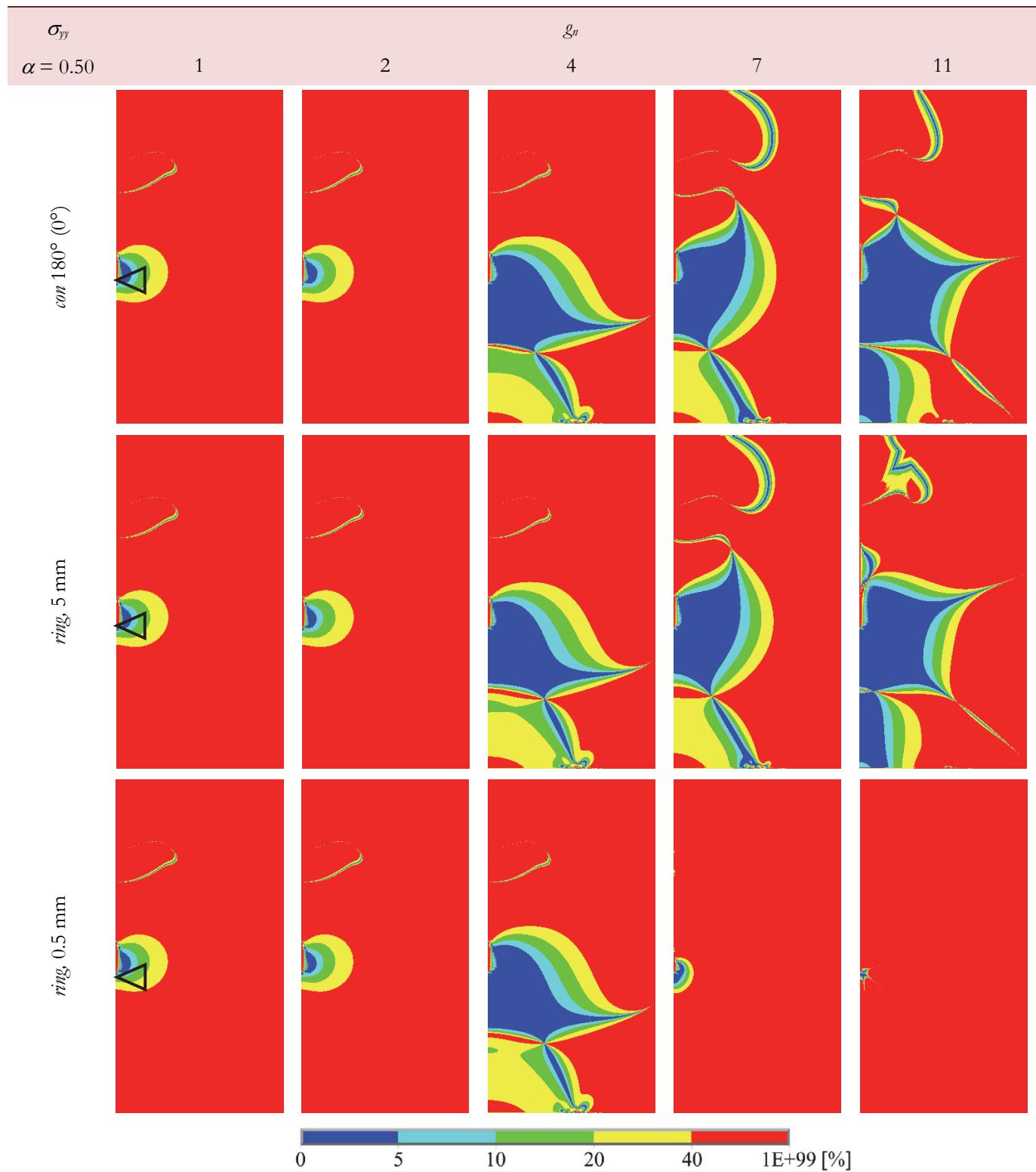
Figure 7: Relative error of crack opening stress  $\sigma_y$  field approximation for chosen variants of nodal selection.
