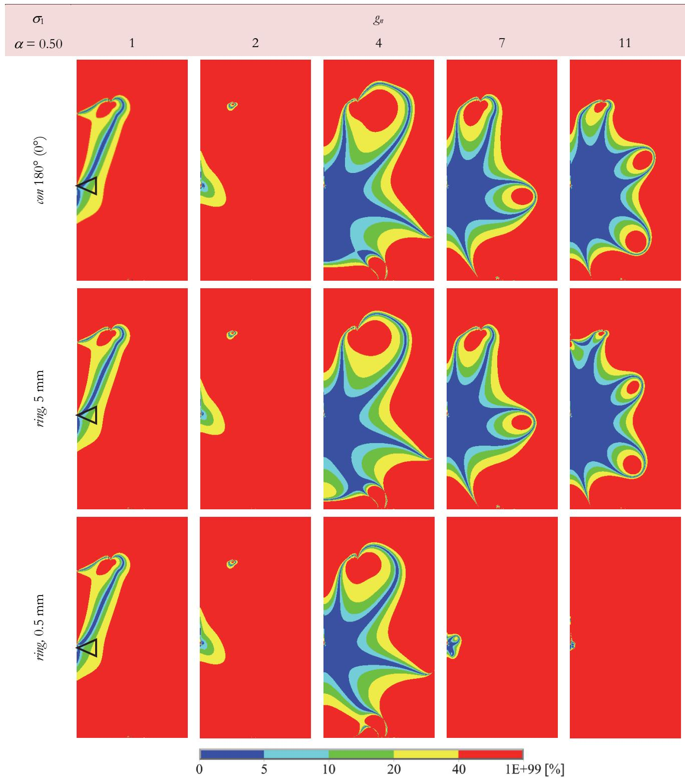
Figure 6: Relative error of principal tensile stress  $\sigma_1$  field approximation for chosen variants of nodal selection.
