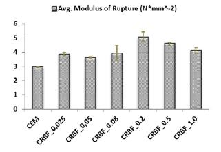
Figure 6: Modulus of rupture of the cement composites with CRBF particles inclusions.
