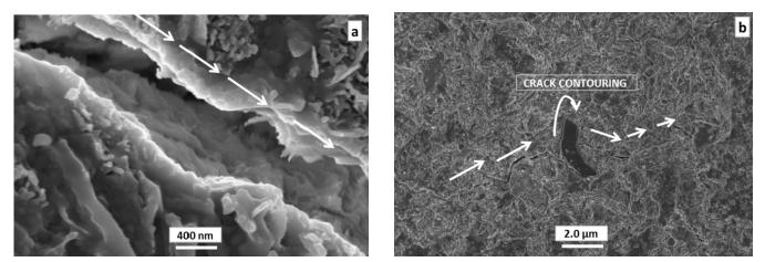
Figure 8: Micro-cracking pattern in plain (a) and CRBF reinforced (b) cementitious composites.
