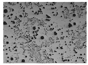
Figure 2: Defects in DCIs. Chunky graphite (x200). Courtesy of Zanardi Fonderie S.p.A.
