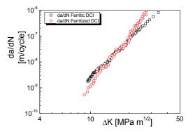
Figure 11: Matrix and loading conditions influence on DCIs ferritic-pearlitic fatigue crack propagation resistance [6].
