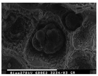
Figure 20: SEM observation of the fracture surface (after overloads).
