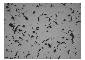
Figure 3: Defects in DCIs. Compacted graphite (x100). Courtesy of Zanardi Fonderie S.p.A.
