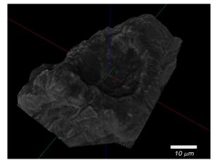
Figure 17: Ferritized DCI. SEM fracture surface analysis: 3D reconstruction ( $\Delta K = 15 \text{ MPa}\sqrt{m}$ ).
