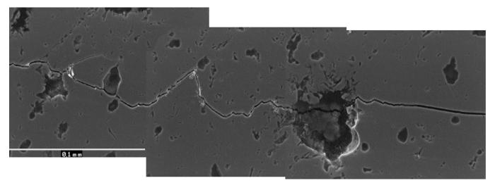
Figure 13: Ferritized DCI. Crack path.
