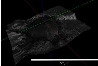
Figure 16: Ferritized DCI. SEM fracture surface analysis: 3D reconstruction ( $\Delta K = 14 \text{ MPa}\sqrt{m}$ ).
