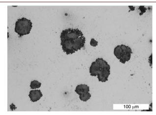
Figure 8: Pearlitic DCI after long annealing heat treatment (ferritic matrix and degenerated graphite elements).
