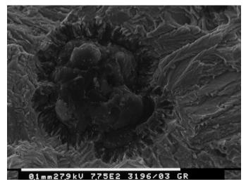
Figure 14: Ferritized DCI. SEM fracture surface analysis ( $\Delta K = 12 \text{ MPa}\sqrt{m}$ ).
