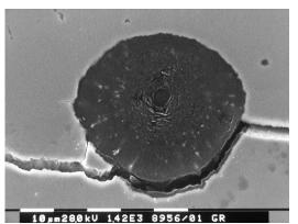
Figure 5: Graphite core-graphite-shield debonding (with residual
