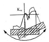
Figure 9: Eucentric tilting.
