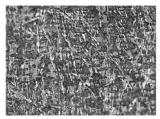
Figure 4: Defects in DCIs. Carbides (x200). Courtesy of Zanardi Fonderie S.p.A.
