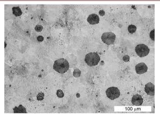
Figure 7: Pearlitic DCI before long annealing heat treatment.
