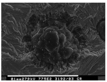
Figure 15: Ferritized DCI. SEM fracture surface analysis ( $\Delta K = 16 \text{ MPa}\sqrt{m}$ ).
