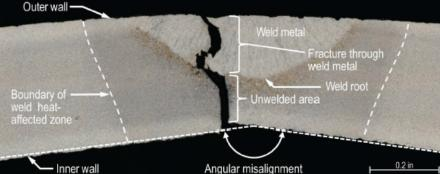
Figure 3: Metallographic image from NTSB Final Report (Fig. 19a) that shows the single-side weld in Pup 1.
