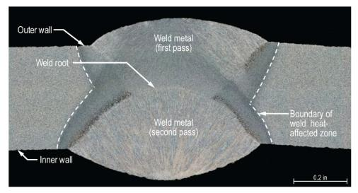
Figure 2: Metallographic cross section of a proper DSAW weld from NTSB Final Report, Fig. 19b.
