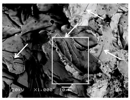
Figure 6: Exponent SEM image of brittle cleavage fracture morphology in Pup 1 final rupture zone. Representative river patterns associated with cleavage fracture are indicated by arrows.
