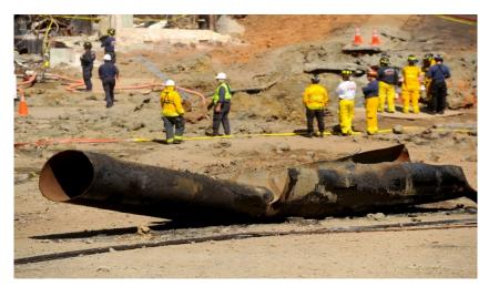
Figure 1: Photograph taken the day after the incident showing the ruptured segment of Line 132 that was ejected from the ground by the force of the rupture. Source: www.dailyrepublic.com.
