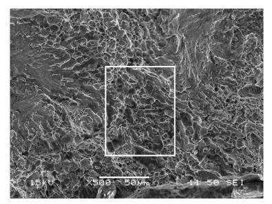
Figure 5: Exponent SEM image that shows microvoid coalescence fracture morphology within the ductile tear (the yellow area in Fig. 3). Representative microvoid coalescence morphology is indicated within the white box.
