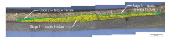
Figure 4: Montage from NTSB Final Report (Fig. 21) that highlights approximate ductile tear (yellow) and fatigue crack growth (green).
