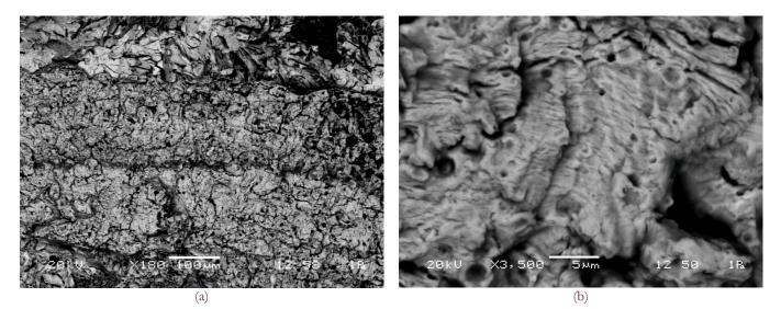
Figure 7: Exponent SEM images: (a) Fatigue striations were observed within Regions A & B, between the ductile tear (Region D) and the final brittle fracture (Region C); (b) Close-up of Region B in image (a), showing representative fatigue striations (within the box).
