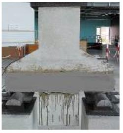
a) CB3u static test without fatigue b) CB3u after one million cycles Figure 8: Cracking and failure in strengthened concrete corbel. a) CB3u-static loading to failure, b) CB3u -after one million cycles.
