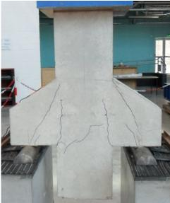
a) "C0" static test without fatigue
