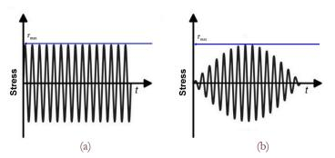
Figure 9: Two different loading paths with same maximum stress.
