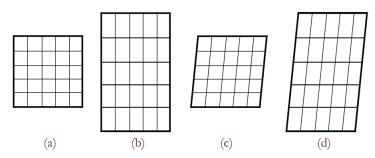
Figure 3: Illustration of different deformation patterns from different loading types. a) Without applied loads, b) axial loading, c) shear loading, and d) biaxial loading.
