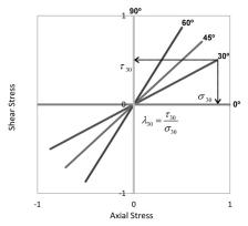
Figure 7: Loading paths used in experiments to calculate the SSF damage function.
