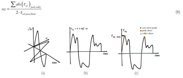
Figure 10: Virtual cycle counting variables identification.
