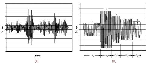
Figure 8: Variable amplitude loadings, a) Time history, b) Equivalent stress spectrum.
