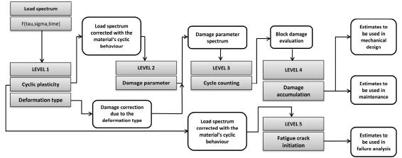
Figure 2: Fatigue estimates process under random loading conditions.
