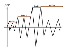
Figure 11: Block extraction methodology for random loadings.
