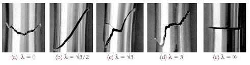
Figure 4: In-phase fracture appearance under different stress amplitude ratios [11].
