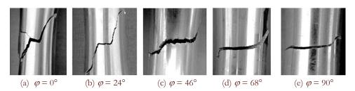
Figure 5: Out-of-phase ( $\phi$ ) fracture appearance for a constant stress amplitude ratio,  $\sqrt{3}$  [11].
