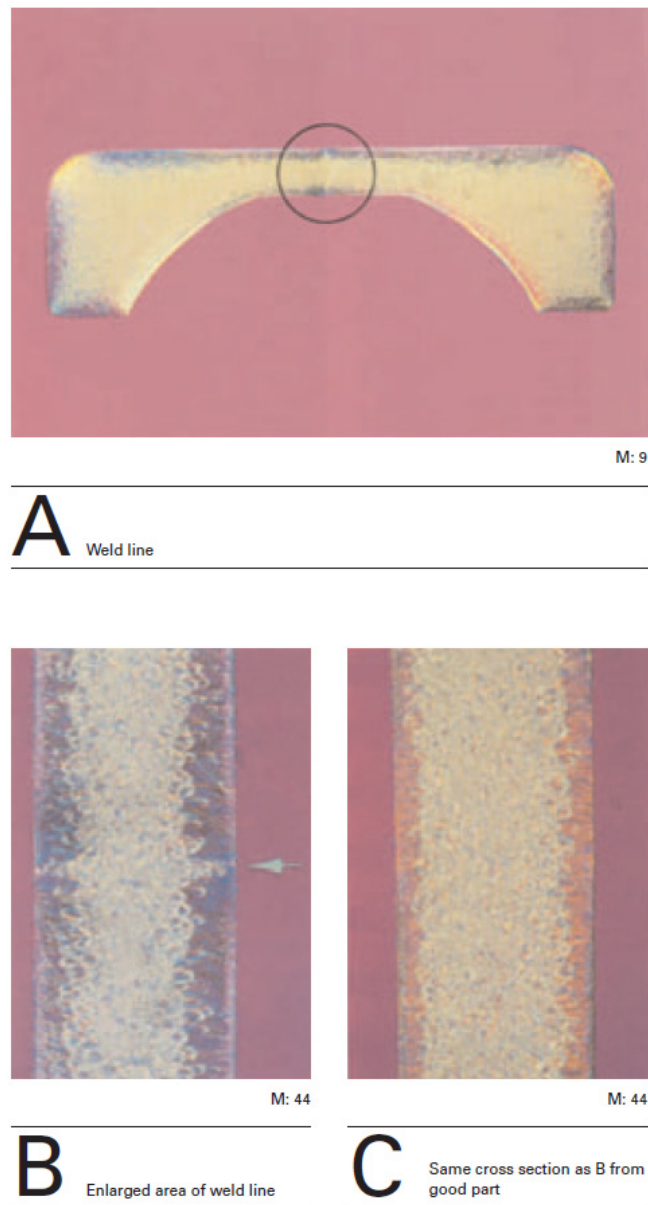
Figure 14. Weld line in a plastic component. [41]
