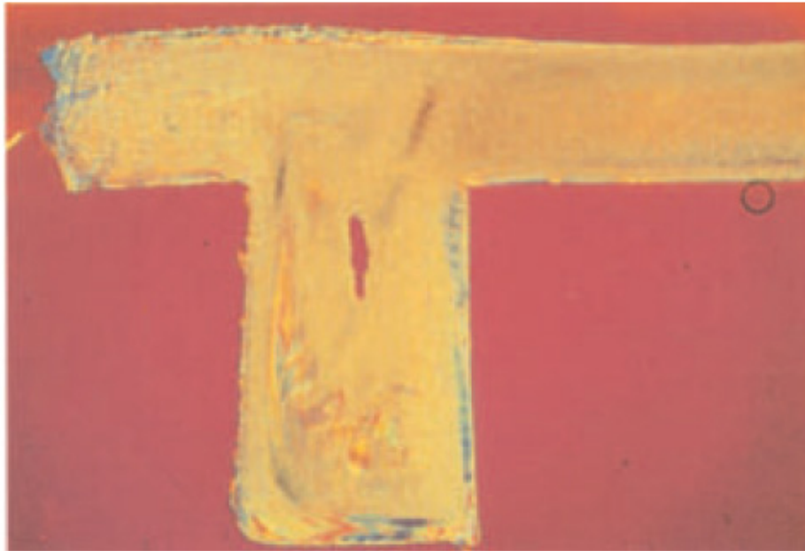
Figure 15. Void and inhomogeneous melt in a plastic component.[41]
