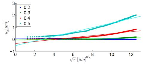
Figure 10: Variations of relative displacement  $(u_j)$  with distance from the crack tip (r) at four different values of load  $(P/P_{max})$  during the initial loading phase of a single cycle. A line of best fit produced with a least squares method is included for each load in the matching colour.
