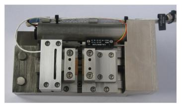
Figure 2: Deben In-Situ Microtest tensile & compression stage with a 2 kN load cell.
