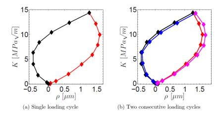
Figure 9: Variation of K and  $\rho$  for loading cycles. Loading phase [black] and unloading [red] are shown for the first cycle. In Fig. 9b a second cycle of loading [blue] and unloading [magenta] is included.
