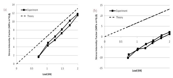
Figure 1: Variation of measured stress intensity factor with load for specimen CTF6 [4] (a) After constant amplitude loading and (b) Immediately after an overload.
