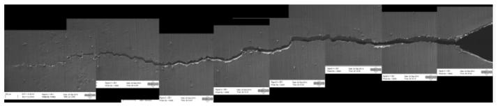
Figure 5: Series of images aligned to give an image of the full crack length at a load of 1:25 kN
