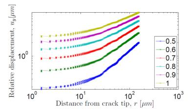
Figure 6: Variation of relative displacement  $(u_y)$  with distance from the crack tip (r) at five different values of load  $(P/P_{max})$  during the loading phase of a loading cycle.
