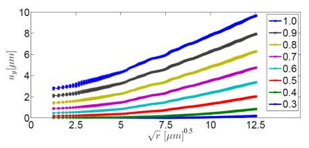
Figure 7: Variations of relative displacement  $(u_y)$  with distance from the crack tip (r) at eight different values of load  $(P/P_{max})$  during the loading phase of a single cycle.
