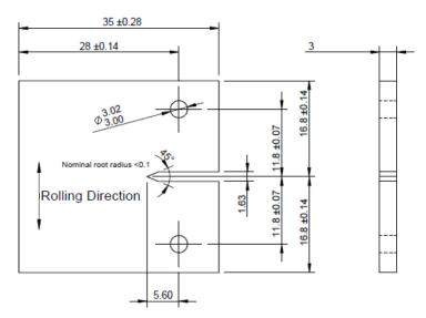
Figure 3: Dimensions (in mm) of specimens used for in-situ SEM testing. Specimens were cut from a sheet of aluminium alloy 6082-T6.
