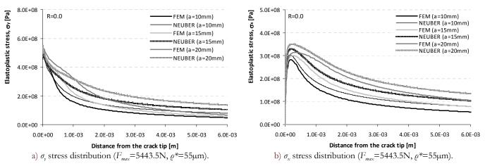
Figure 12: Elastoplastic stress distribution ahead of the crack tip along the crack plane line (y=0) for CT specimens made of S355 steel: comparison between analytical and numerical results. Distinct crack sizes considered.
