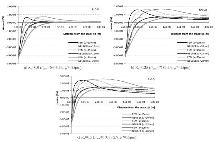
Figure 13: Residual stress distribution ahead of the crack tip along the crack plane line (y=0) for CT specimens made of S355 steel: comparison between analytical and numerical results. Distinct stress ratios and crack sizes considered.
