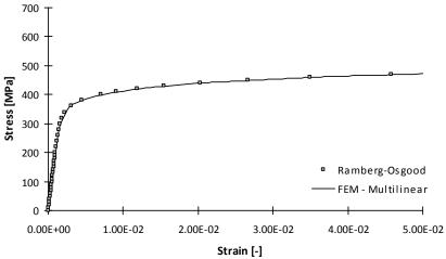
Figure 9: Cyclic curve of the S355 steel.
