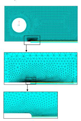
Figure 8: Typical finite element mesh of the CT specimen, using 6-noded quadratic triangular plane stress elements.
