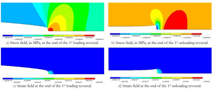
Figure 14: Stress and strain fields, along the load direction, obtained for the CT specimens made of S355 steel, resulting from elastoplastic finite element analysis ( $\rho$ \*=55µm, a=15mm,  $R_{\sigma}$ =0.0,  $F_{max}$ =5443.5N).
