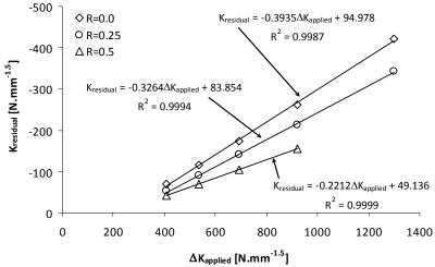
Figure 15: Residual stress intensity factor as a function of the applied stress intensity factor range obtained for the S355 steel  $(e^*=5.5\times10^{-5}\text{m})$ .
