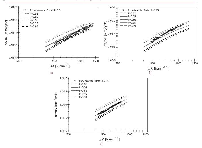
Figure 17: Probabilistic prediction of the fatigue crack propagation based the *p-SWT-N* field, for the S355 steel: a)  $R_{\sigma}$ =0; b)  $R_{\sigma}$ =0.25; c)  $R_{\sigma}$ =0.5.
