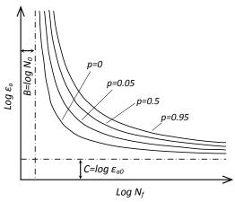
Figure 2: Percentile curves representing the relationship between dimensionless lifetime,  $N_i^*$ , and the strain amplitude,  $\varepsilon_a^*$ : p- $\varepsilon_a$ -N field.
