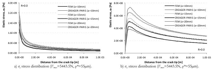
Figure 11: Elastic stress distribution ahead of the crack tip and along the crack plane line (y=0) for CT specimens made of the S355 steel: comparison between analytical and numerical results. Distinct crack sizes considered.
