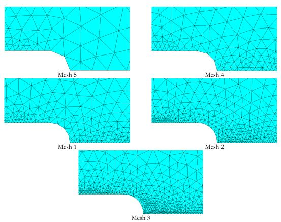
Figure 10: Finite element meshes used in the convergence study for the S355 steel ( $\rho = 55 \mu m$ ).
