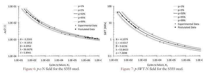
The *p-ɛ-N* and *p-SWT-N* fields of the S355 steel are presented in Figs. 6 and 7, respectively. The constants of the Weibull fields are also referred in the figures. The extrapolations using the Weibull field should be avoided for high- and low-cycle fatigue lives. Since the number of cycles to fail the representative volume element, in the crack propagation regime, may
