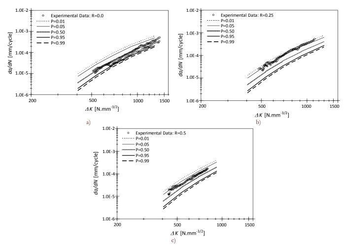
Figure 16: Probabilistic prediction of the fatigue crack propagation based the *p-\varepsilon-N* field, for the S355 steel: a)  $R_{\sigma}$ =0; b)  $R_{\sigma}$ =0.25; c)  $R_{\sigma}$ =0.5.
