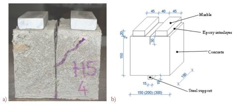
Figure 1: Wedge splitting specimen: a) photo and b) sketch: where the rectangular groove is formed by two marble plates glued on the upper side of the specimen.
