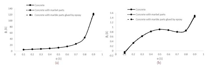
Figure 5: The values of normalized stress intensity factor  $B_1$  and T-stress  $B_2$  for W = 150 mm for three cases: i) concrete (E = 40 GPa), ii) concrete (E = 1 GPa) with marble parts (E = 100 GPa) and iii) concrete (E = 100 GPa) with marble parts (E = 10 GPa) glued by epoxy (E = 5 GPa).
