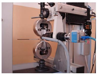
Figure 3: DBC test apparatus with CCD camera video image.
