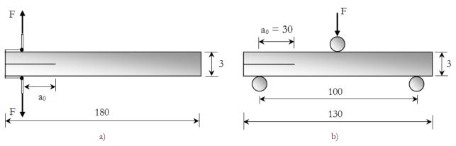
Figure 2: a) DCB specimen (Mode I); b) ENF specimen (mode II). Dimensions in mm.
