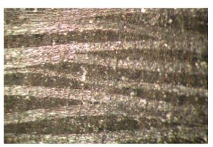
Figure 1: Lateral view photo showing the fibre distribution along of the longitudinal direction of the specimen.
