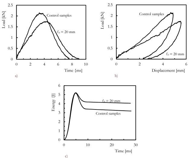
Figure 3: Comparison of the gap's effect in terms of a) load-time curves; b) load-displacement curves; c) energy-time curves.
