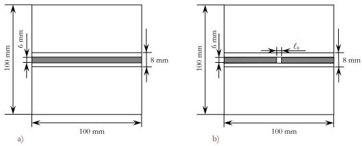
Figure 1: a) Control samples; b) Samples with different gap lengths ( $\ell_0 = 20$  mm).
