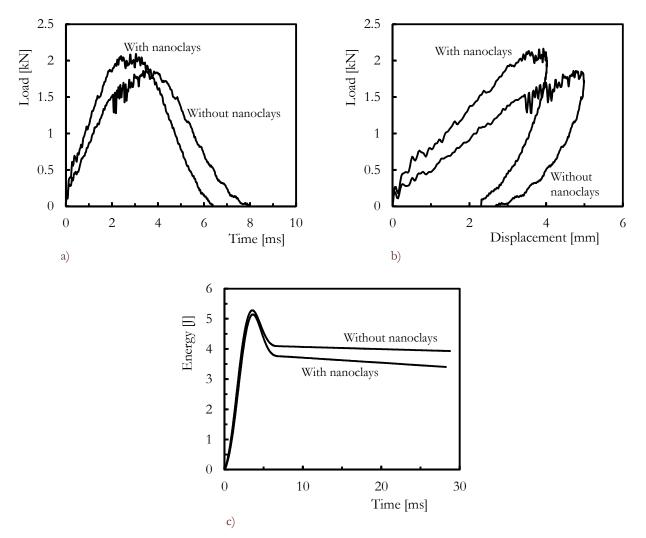
Figure 2: a) Typical load-time curves; b) Typical load-displacement curves; c) Typical energy-time curves.
