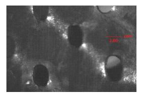
Figure 11: Shear band formation during the tensile deformation of specimen (For Hole orientation (i) 60° and strain at 16%, (ii) 45° and strain at 18 % respectively).
