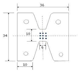
Figure 3: Square specimen with array of hole.
