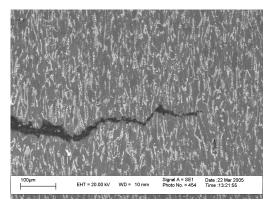
Figure 12: Fracture path under Microscope.
