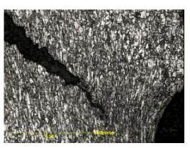
Figure 13: Grain in front of crack tip.
