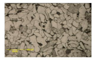
Figure 9: Void nucleation at grain boundary.
