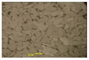
Figure 8: Structure of undeformed specimen.
