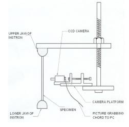
Figure 5: CCD camera stage
