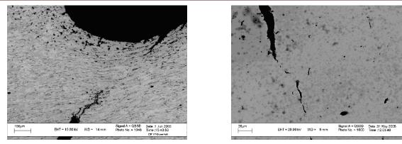
Figure 16: Void coalescence in front of crack.
