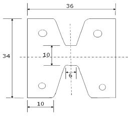
Figure 2: Flat square specimen (thickness 1mm.)
