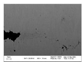
Figure 15: Void coalescence in front of crack.
