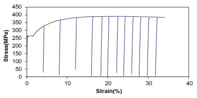
Figure 6: Stress-strain curve obtained during the loading and unloading operation for the flat tensile specimen.
