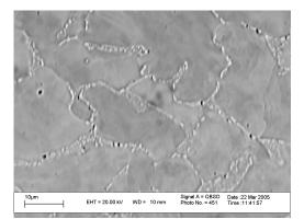
Figure 14: Voids present at grain boundary.
