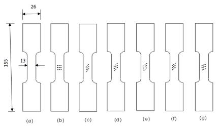
Figure 1: Rectangular specimen with arrays of holes at different orientations: (a) Specimen without hole, (b) hole array at 00/900, (c) at  $30^{\circ}$ , (d) at  $40^{\circ}$ , (e) at  $45^{\circ}$ , (f) at  $50^{\circ}$  and (g) at  $60^{\circ}$ .
