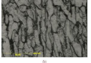
Figure 10: Elongated grain at (a) 20% strain and (b) 40% strain. (The tensile load axis is horizontal and vertical respectively for the above figures).
