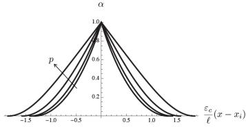
Figure 4: Damage profile in the localization zone when the bar breaks, for q = 4 and different values of the parameter p (p = 1/2, 1, 2, 4) in the family of brittle materials of Example 1.
