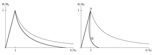
Figure 7: Overall stress-strain relations for a law of Example 2 with p = 4 and q = 2 (Thin curve=homogeneous response; Thick curve=localized response). Left: For a bar of intermediate length; Right: For a long bar.
