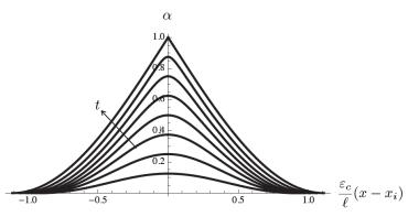
Figure 5: The damage profile for a given t and its evolution with t by assuming that  $t \mapsto \sigma_t$  is decreasing in the case of the model of Example 1 with p = 2 and q = 4. The rupture occurs when  $\sigma_t = 0$  and  $\overline{\alpha}(\sigma_t) = 1$ . We check numerically that  $\sigma \mapsto D(\sigma)$  is decreasing.
