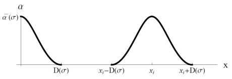
Figure 2: A typical damage profile in an inner localization zone and in a boundary localization zone when  $0 \le \sigma \le \sigma_c$
