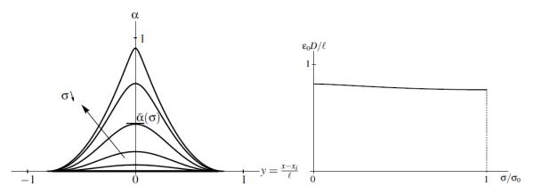
Figure 3: Left: The damage profile for a given  $\sigma$  and its evolution for different  $\sigma$  in the case of the model of Example 2 with q = 2and p = 4 (the lower  $\sigma$ , the higher  $\alpha$ ). Right: We check numerically that  $\sigma \mapsto D(\sigma)$  is decreasing.
