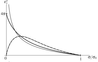
Figure 6: Graph of the function  $\sigma \mapsto \varepsilon_1^d(\sigma)$  giving the contribution of a localized zone on the overall strain in the case of the model of Example 2 with p = 4 and different values of q (dashed: q = 1, thick: q = 2, thin: q = 3).
