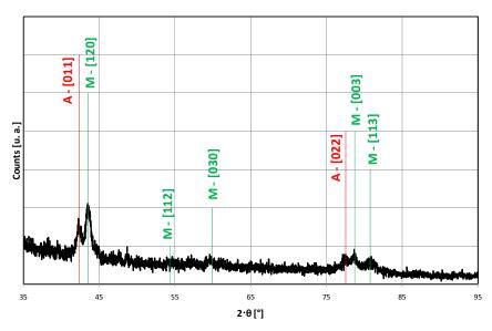
Figure 11: X-Ray spectra of obtained from unloading from  $\varepsilon_g$ =10% to  $\varepsilon_g$ =5%.
