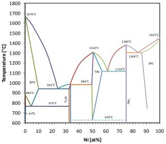
Figure 1: NiTi alloy phase diagram.
