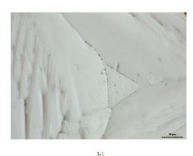
Figure 2: Initial austenitic microstructure of the investigated NiTi alloy: a) at low magnification showing the presence of inclusions, b) high magnification with presence of subgrains.
