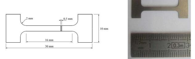
Figure 4: Uniaxial miniaturized specimens.
