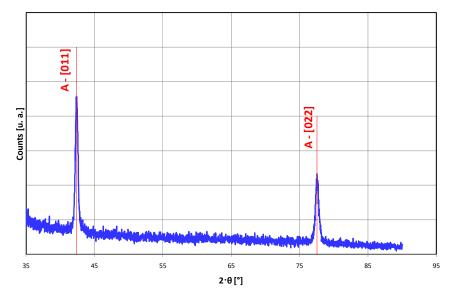
Figure 8: X-Ray spectra of the investigated NiTi alloy in stress free condition.
