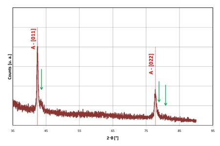
Figure 9: X-Ray spectra obtained from monotonic loading up to  $\varepsilon_g$ =5%.
