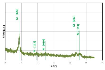
Figure 10: X-Ray spectra obtained from monotonic loading up to  $\varepsilon_g$ =10%.
