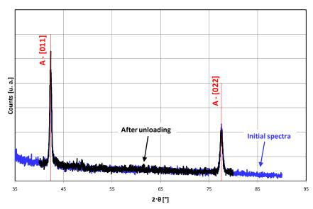
Figure 12: Comparison of the X-Ray spectra between initial condition and final stress free condition after unloading.
