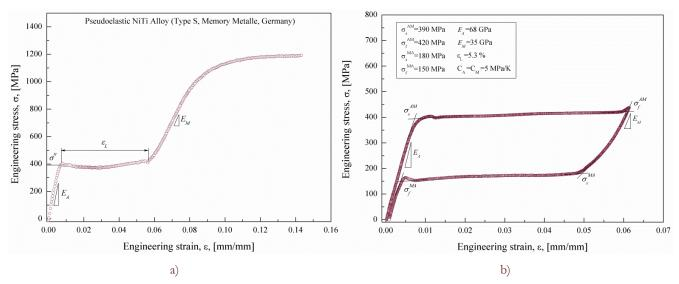
Figure 3: Isothermal stress-strain curve of the investigated alloy carried out at room temperature (T=298k): a) monotonic loading to fracture and b) loading-unloading cycle.
