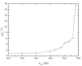
Figure 3: Temperature increment at different stress amplitude.
