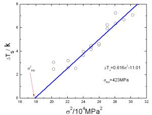
Figure 5: Fatigue limit stress by the infrared thermographic method.
