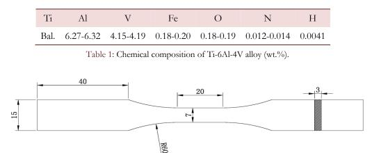
Figure 1: Size of the specimen (unit: mm).
