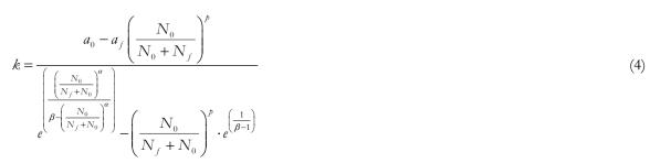
and where  $a_0$  and  $a_f$  are respectively the initial and final crack lengths, N<sub>f</sub> is the number of cycles to failure and  $N_0$ ,  $\alpha$ ,  $\beta$  and p are four parameters to be determined by least-square method.
