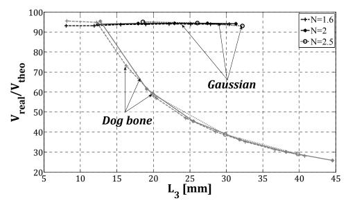
Figure 4: Percent ratio  $V_{\it real}$  /  $V_{\it theor}$  in dog-bone and Gaussian specimens with respect to the length  $L_3$  .
