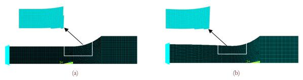
Figure 2: Typical mesh for the specimen models: (a) dog-bone specimen; (b) Gaussian specimen.
