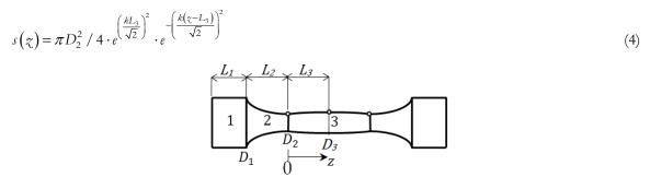
Figure 1: Gaussian specimen.
