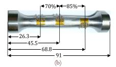
Figure 6: Specimens after application of strain gage rosettes: (a) dog-bone shaped specimen; (b) Gaussian specimen.
