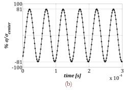
Figure 7: Stress variation measured by strain gage rosettes bonded to the dog-bone shaped specimen: (a) rosette at 70% of  $L_3$ ; (b) rosette at 85% of  $L_3$ .
