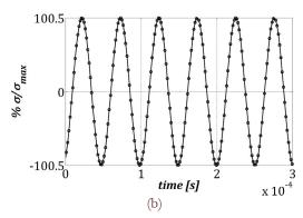
Figure 8: Stress variation measured by strain gage rosettes bonded to the Gaussian specimen: (a) rosette at 70% of  $L_3$ ; (b) rosette at 85% of  $L_3$ .
