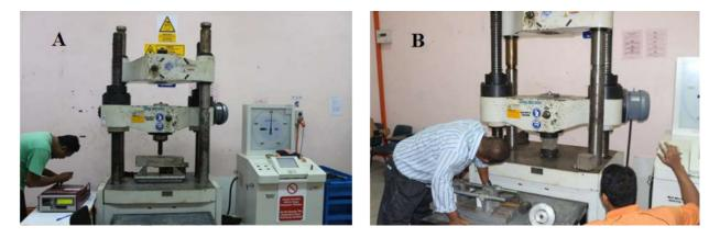
Figure 5: Deflection testing equipment for testing beam B1 (part A) and same equipment used to measured compressive strength of plain concrete cube (part B).
