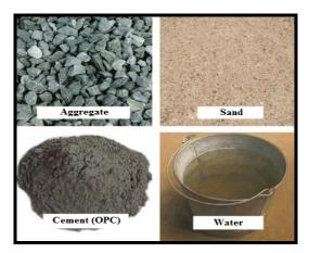
Figure 3: Basic materials of concrete.
