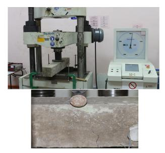
Figure 14: Failure mode for beam B2, non-fiber reinforced Figure 15: Failure mode for beam B2, content 1.0% steel fibers. concrete.
