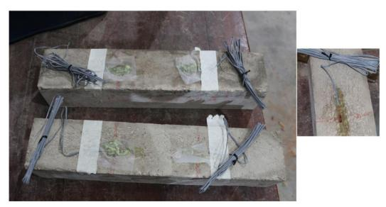
Figure 7: Strain gauges installed on concrete beam.
