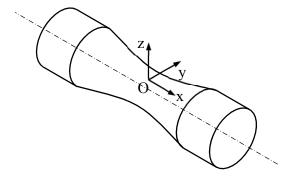
Figure 2: Cylindrical specimen and adopted frame of reference.
