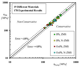
Figure 5: Accuracy of the MWCM, applied in terms of nominal stresses, in estimating high-cycle fatigue strength of notched metallic materials subjected to multiaxial loading paths, where IPh=in-phase, OoPh=out-of-phase, ZMS=zero mean stress, N-ZMS=non-zero mean stress.
