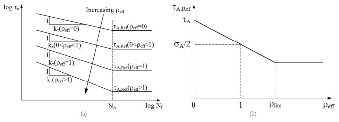
Figure 1: Modified Wöhler diagram (a) and adopted correction for the  $\tau_{A,Ref}$  vs.  $\rho_{eff}$  relationship (b).
