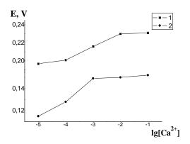
Figure 1. Dependence of the equilibrium potential of the plasticized electrode on concentration of  $Ca^{2+}$ : 1 – Type 1 electrode (untreated); 2 – Type 2 electrode (pretreated).
