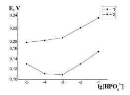
Figure 2. Dependence of the equilibrium potential of the electrode on concentration of  $HPO_4^{2^-}$ : 1 – Type 1 electrode (untreated); 2 – Type 2 electrode (pretreated in the 10<sup>-3</sup> mol/dm<sup>3</sup> solution of Ca(NO<sub>3</sub>)<sub>2</sub>).
