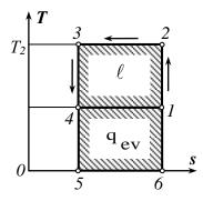
Fig. 2. Diagram of the system with mechanical compression of the secondary steam in coordinates T-s
