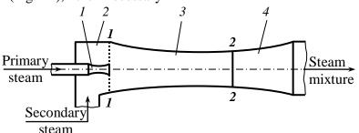
Fig. 4. Scheme of the ejection thermocompressor: 1 - working nozzle; 2 - receiving camera; 3 - mixing chamber; 4 - diffuser
