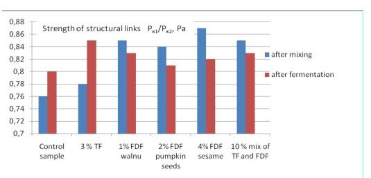
Fig. 3. Influence of TF and FDF on strength of structural links
