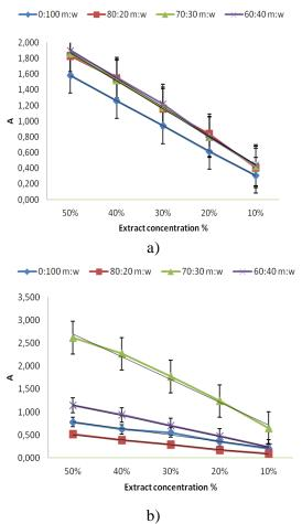
Fig. 2. Absorbance curves for extracts diluted with aqueous methanol solutions (0:100, 60:40, 70:30 and 80:20, methanol: distillated water) from: a) white seeds; b) red seeds
