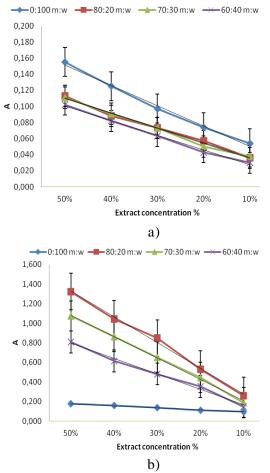
Fig. 1. Absorbance curves for extracts diluted with aqueous methanol solutions (0:100, 60:40, 70:30 and 80:20, methanol: distillated water) from: a) white peels; b) red peels
