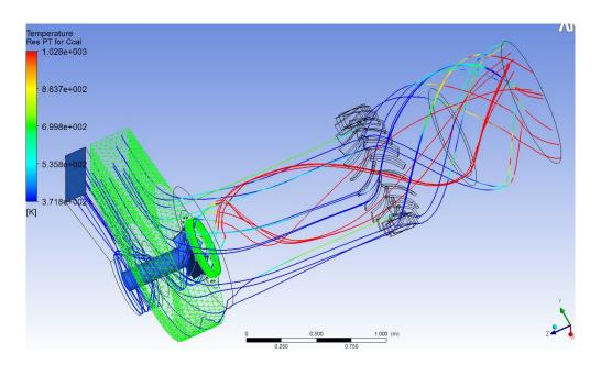
Fig.8.3-D coal particles tracks (coloured by temperature).
