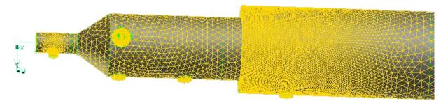
Fig. 2.The image of the VGP unit outer surface partition on computation mesh
