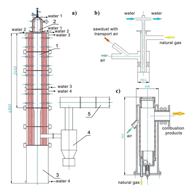
Fig. 1. VGP-100B unit geometry: a) VGP-100B experimental unit (1 – reactor diagnostic area; 2 – burner device; 3 – slag collector; 4 – cyclone; 5 – cooling chamber);b) primary burner; c) auxiliary burner
