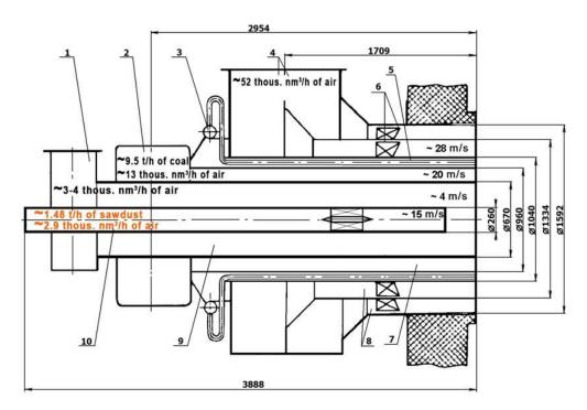
Fig. 9. Boiler unit TPP-210A burner retrofit for co-combustion:
