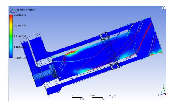
Fig.7. The volatiles concentration field in burner cross section combined with coal particles' tracks (coloured by temperature).
