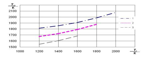
Fig. 4. Calculated values of the unsheathed thermocouple readings in flue gases with irradiating to cooled walls at *Tc* at different temperatures of flow :  $1 - T_e = 2200 [K]; 2 - T_e = 2000 [K]; 3 - T_e = 1800 [K].$
