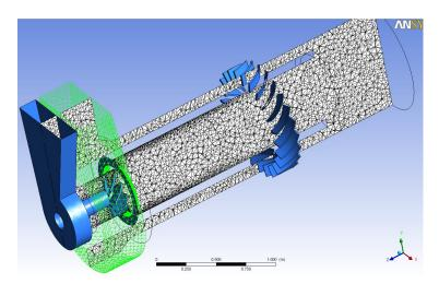
Fig. 5. The burner mesh of the TPP-210A boiler
