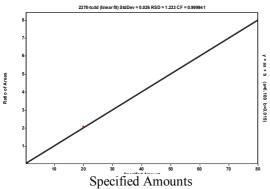
Figure 1. Calibration curve for 2378-TetraCDD
