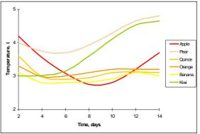
Figure 2. The variation of bulk fruits' core temperature at refrigeration
