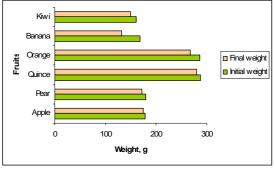
Figure 3. The water losses variation during refrigeration of bulk fruits
