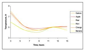
Figure 1. The cooling rate of the bulk fruits at refrigeration
