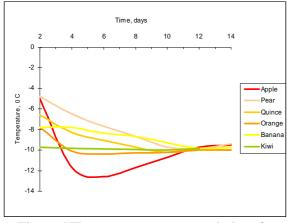
Figure 6 The core temperature variation of freeze bulk fruits
