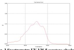
Fig. 3-Spectrometry UV-VIS  $\beta$  carotene absolute (Merck) ethalon
